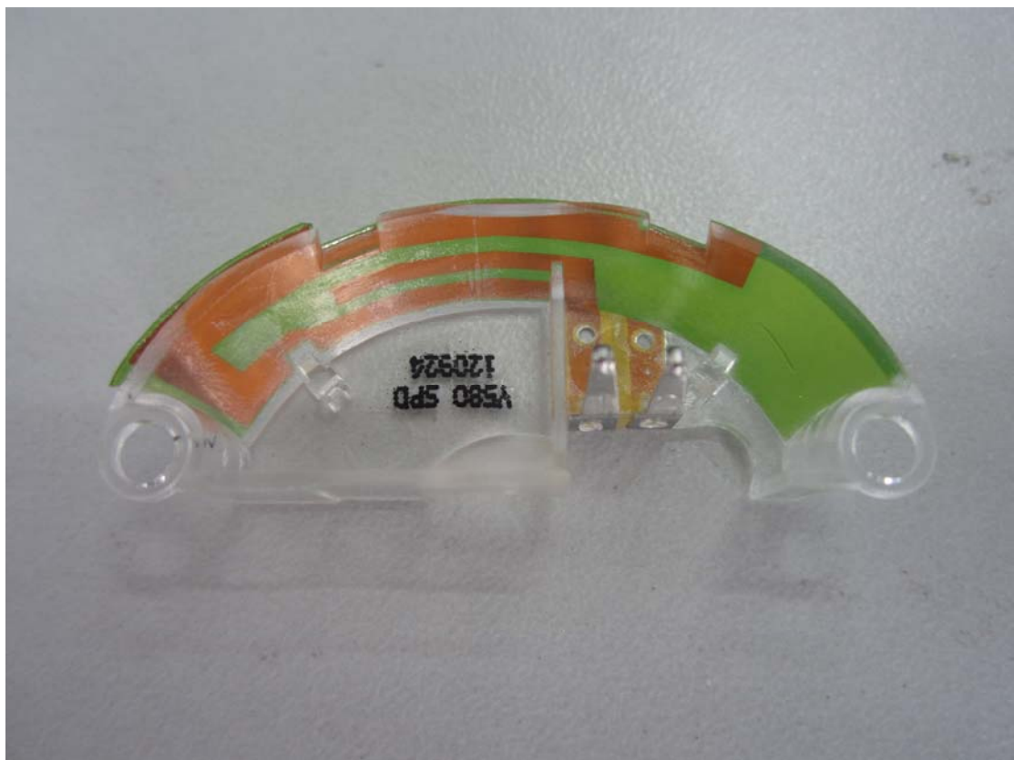
10. WIFI antenna view
