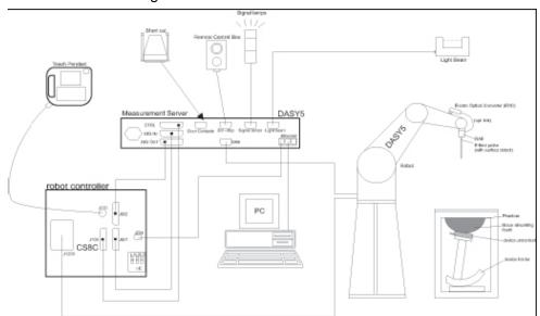
Picture C.1 SAR Lab Test Measurement Set-up
