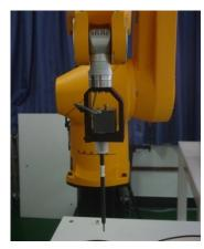
Picture C.3 E-field Probe
