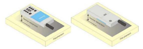
Picture D.4 Test positions for body-worn devices
