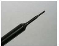
Picture C.2 Near-field Probe
