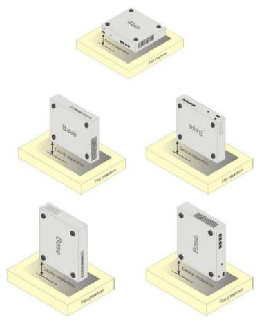
Picture D.5 Test positions for desktop devices
