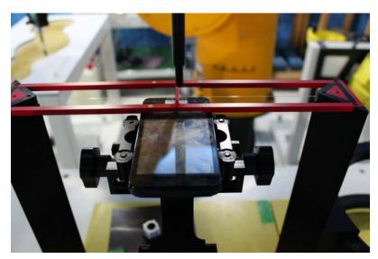
Picture 2: EUT Positioning for RF
