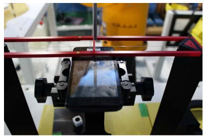
Picture 3: EUT Positioning for T-coil
