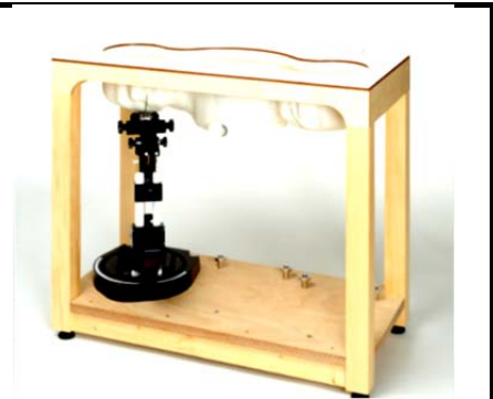
Fig 5.6 Photo of SAM Phantom
