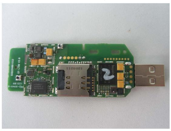
6. Mainboard rear view without shielding
