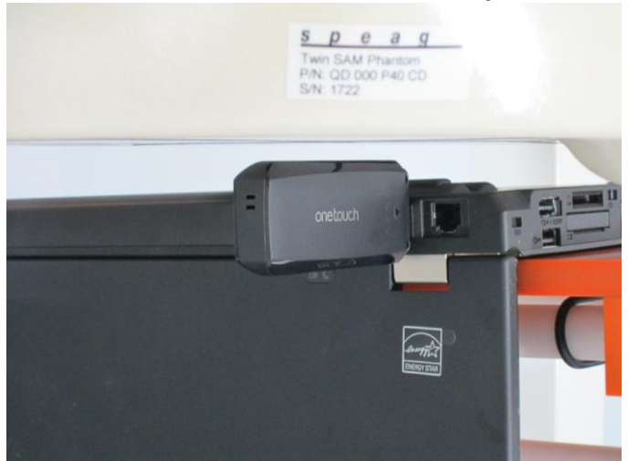
Vertical Back with 5 mm Gap
