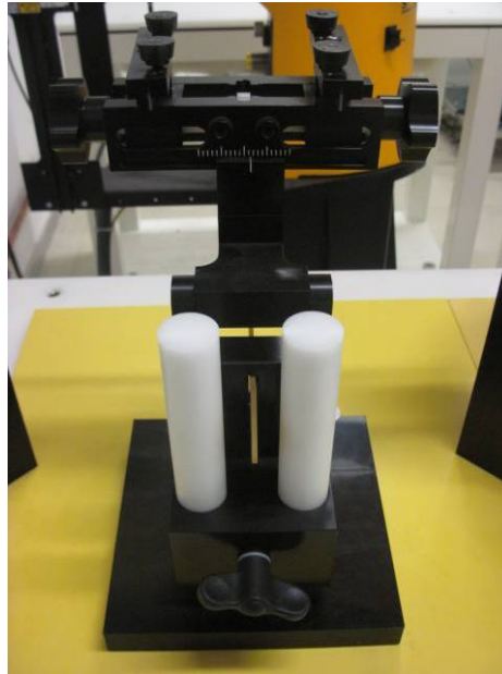
Fig. 2 HAC Phantom & Device Holder
