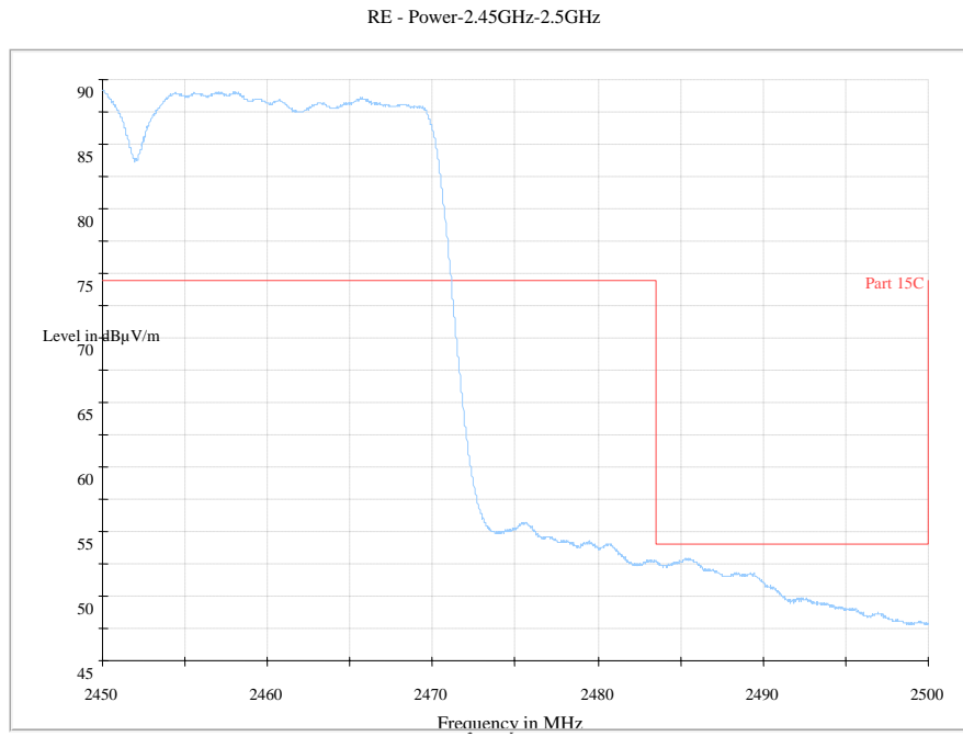
Fig. 169 Radiated Spurious Emission (Power): 802.11n-40MHz, ch9, 2.45 GHz - 2.50GHz
