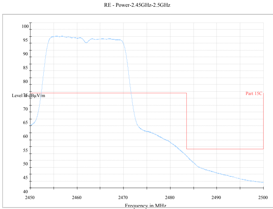
Fig. 147 Radiated Spurious Emission (Power): 802.11g, ch11, 2.45 GHz - 2.50GHz
