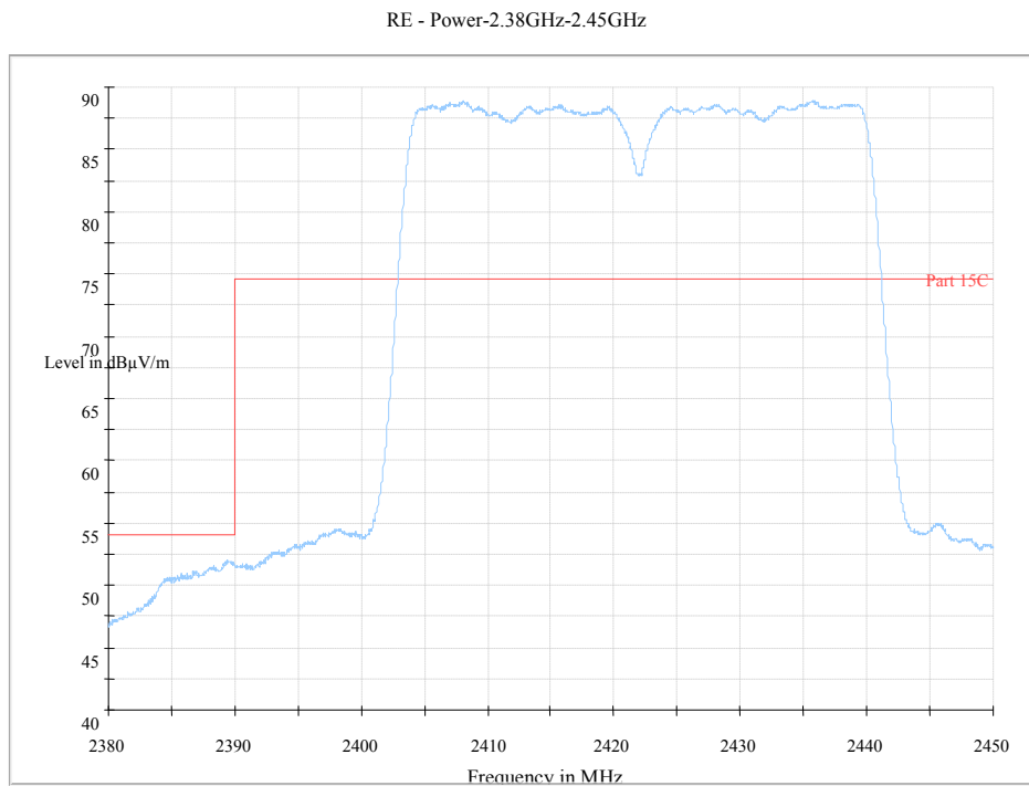
Fig. 162 Radiated Spurious Emission (Power): 802.11n-40MHz, ch3, 2.38 GHz - 2.45GHz
