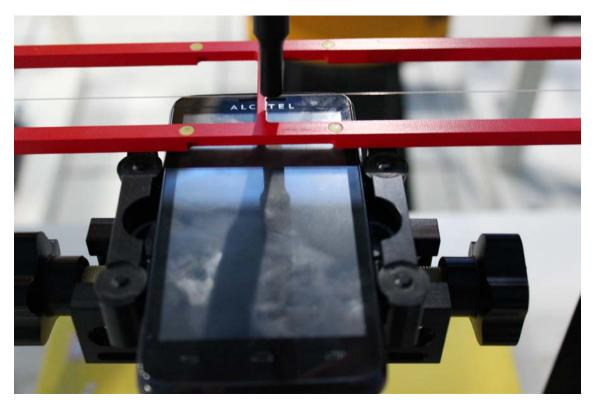
Picture 2: EUT Positioning for RF
