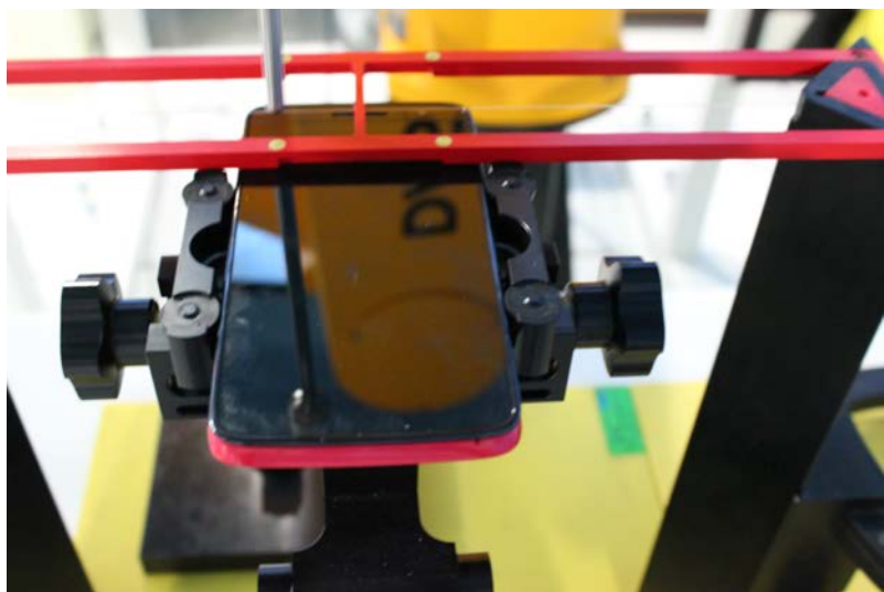
Picture 3: EUT Positioning for T-coil
