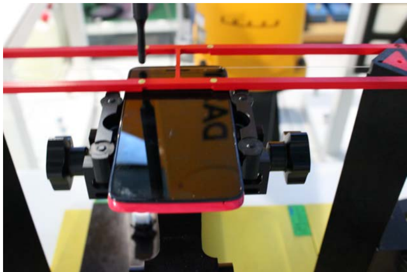
Picture 2: EUT Positioning for RF
