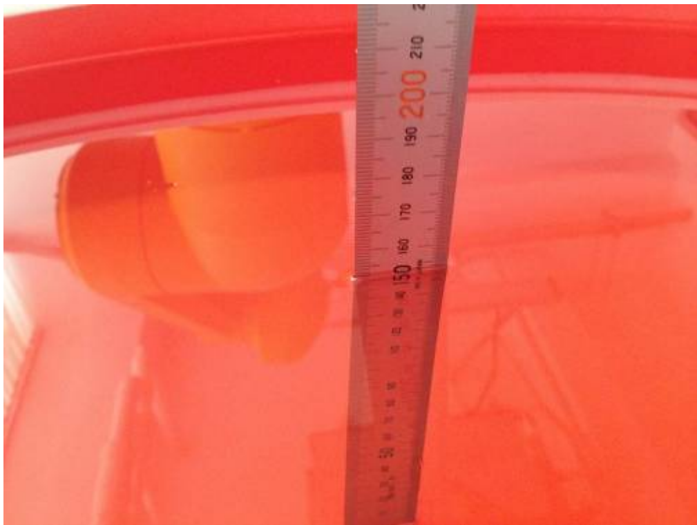
Picture 7-6 Liquid depth in the Flat Phantom (2450MHz)
