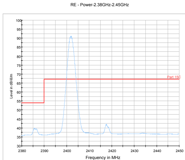
Fig.91. Radiated emission (Power): 8DPSK, low channel
