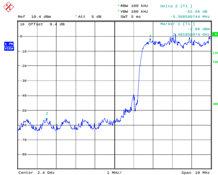
Fig.5. Frequency Band Edges: \pi/4 DQPSK, Channel 0, Hopping Off
