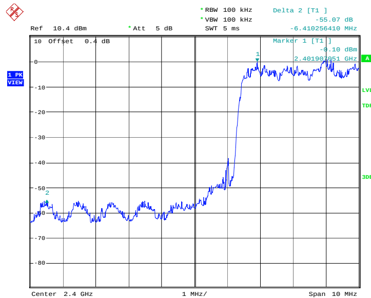
Fig.9. Frequency Band Edges: 8DPSK, Channel 0, Hopping Off
