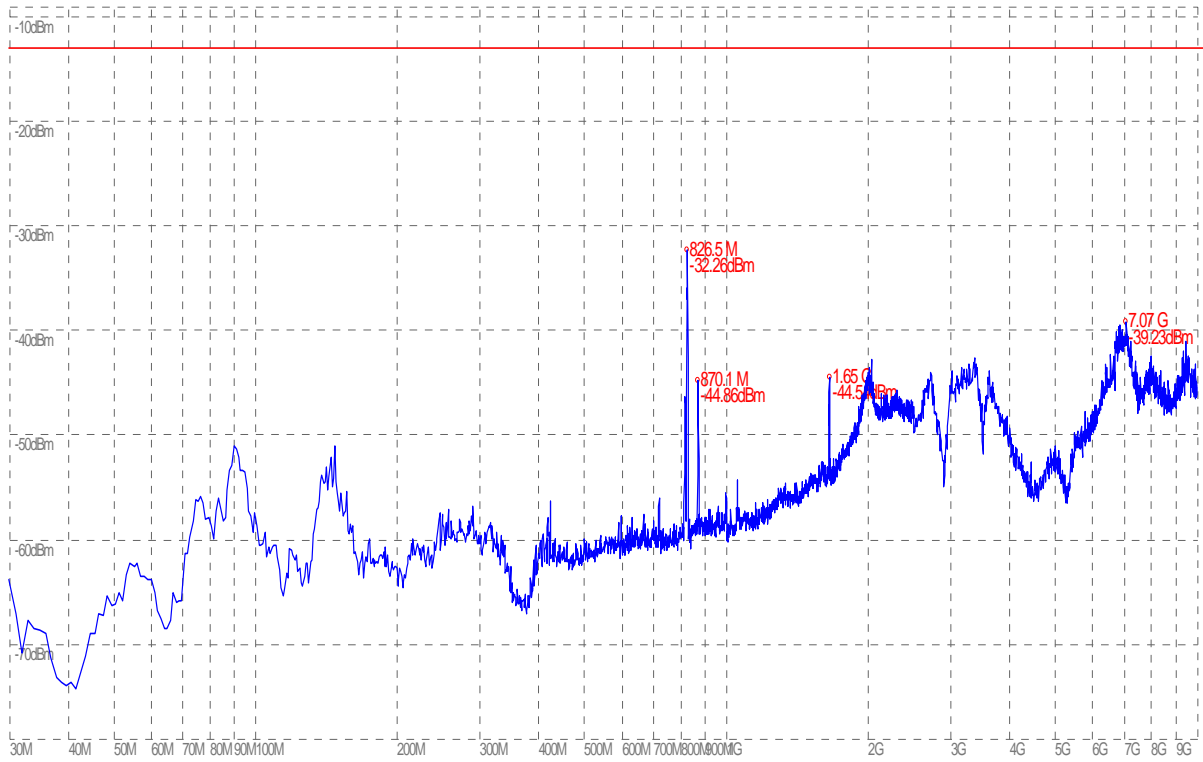
(Plot G.3: HSDPA 850MHz Channel = 4175, Test Antenna Horizontal)
