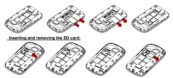
To release the microSD card holder, slide it in the direction of the arrow and lift it. Then insert the microSD card with the golden contact downward. Finally, turn down the microSD holder and slide it in the opposite direction to lock it.
