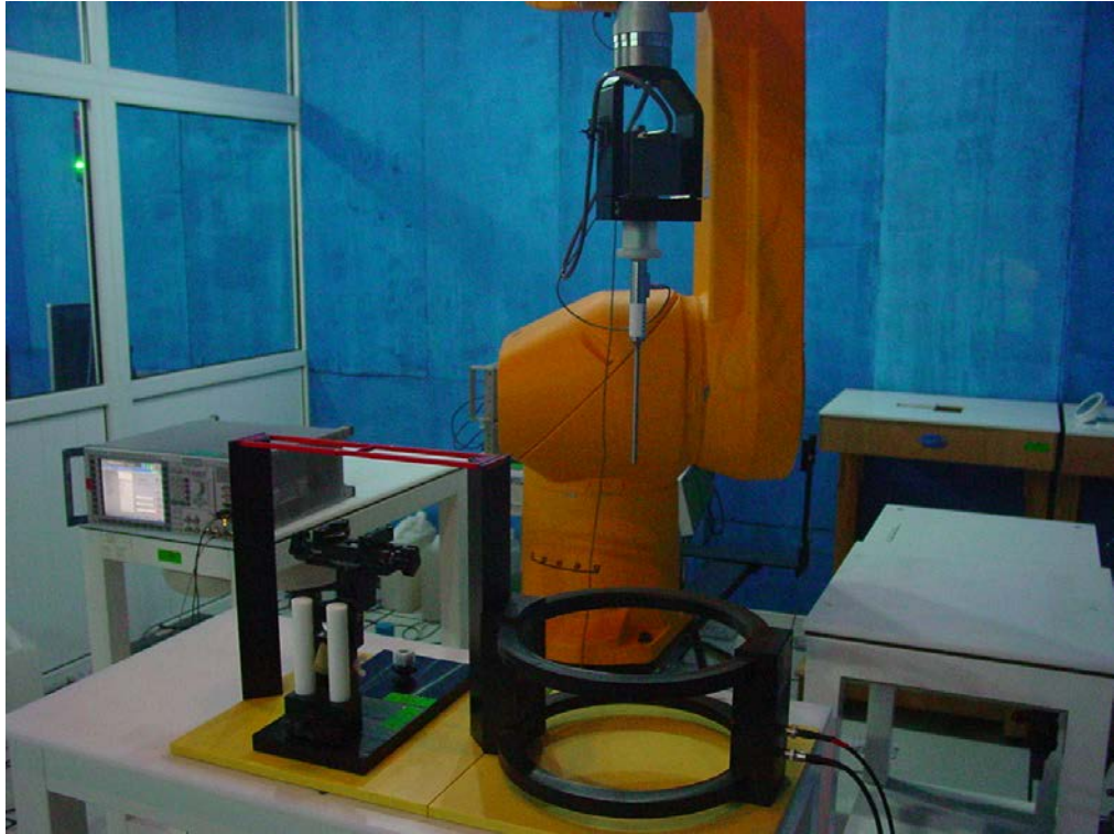
Picture A1: HAC T-Coil System Layout
