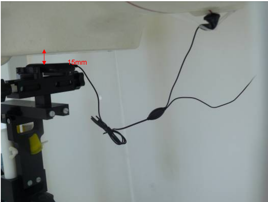
Picture 13: Body with Stereo Headset 1, The EUT display towards ground, the distance from EUT to the bottom of the Phantom is 15mm
