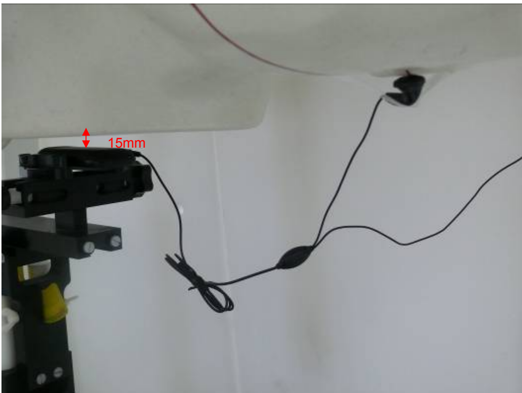
Picture 14: Body with Stereo Headset 2, The EUT display towards ground, the distance from EUT to the bottom of the Phantom is 15mm
