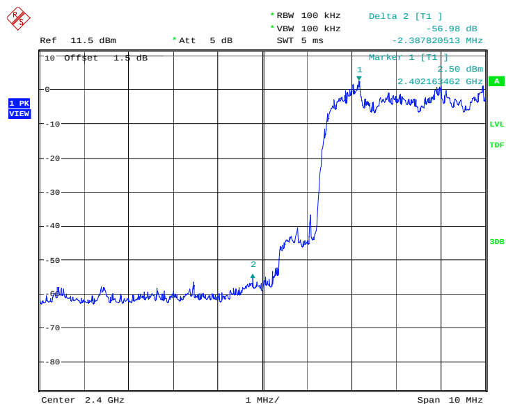
Fig.9. Frequency Band Edges: 8DPSK, Channel 0, Hopping Off
