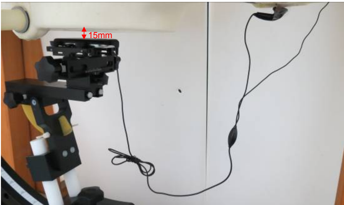
Picture 14: Body with Stereo Headset 2, The EUT display towards ground, the distance from EUT to the bottom of the Phantom is 15mm
