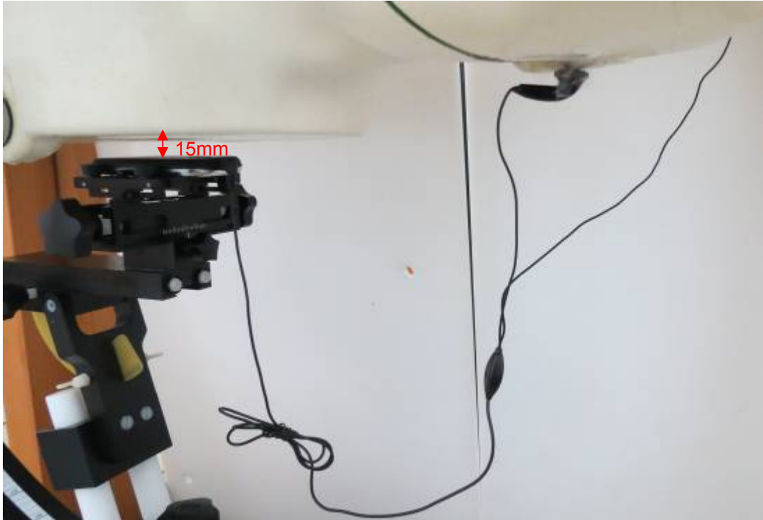
Picture 13: Body with Stereo Headset 1, The EUT display towards ground, the distance from EUT to the bottom of the Phantom is 15mm
