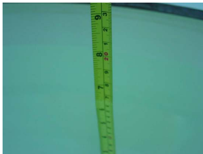
Picture 9.2 Liquid depth in the Flat Phantom (1750MHz)
