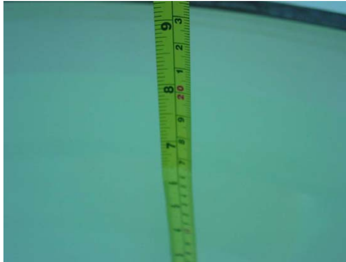
Picture 9.3 Liquid depth in the Flat Phantom (1900MHz)
