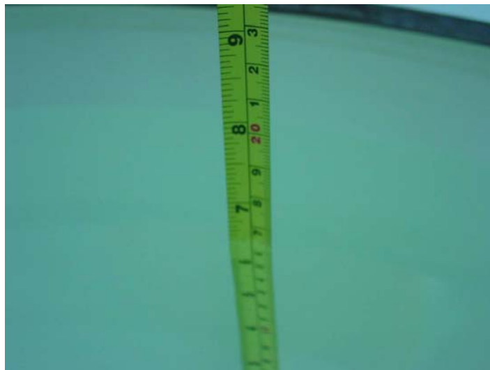
Picture 9.4 Liquid depth in the Flat Phantom (2450MHz)
