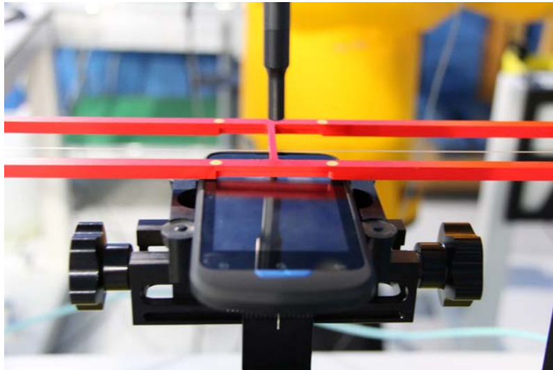
Picture 2: EUT Positioning for RF
