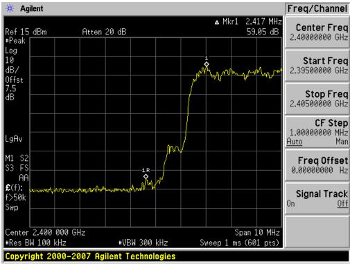
Test Plots with hopping (8DPSK) Band Edges (High-CH)
