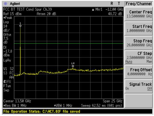
Test Plots (8DPSK) - 1 GHz - 26 GHz (RBW:1 MHz, VBW: 1 MHz) Spurious Emission (High-CH)
