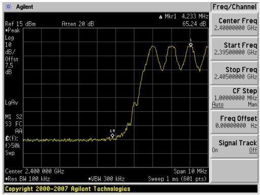
Test Plots with hopping (GFSK) Band Edges (High-CH)
