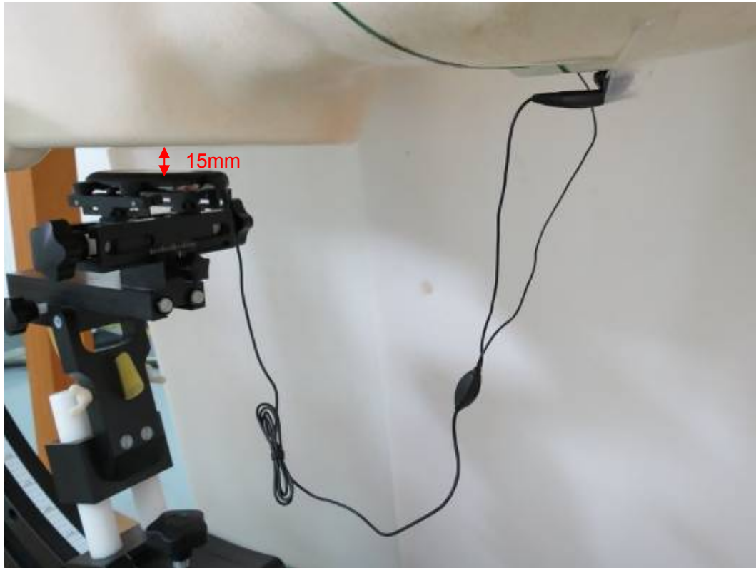
Picture 13: Body with Stereo Headset, The EUT display towards ground, the distance from EUT to the bottom of the Phantom is 15mm
