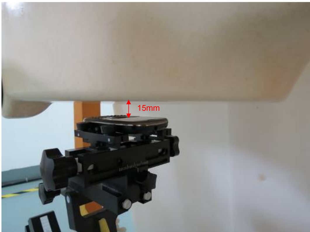
Picture 12: Body, The EUT display towards phantom, the distance from EUT to the bottom of the Phantom is 15mm
