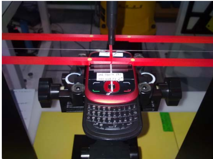
Picture 2: EUT Positioning for RF
