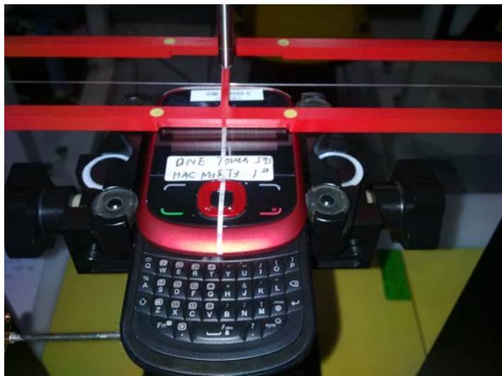
Picture 3: EUT Positioning for T-coil
