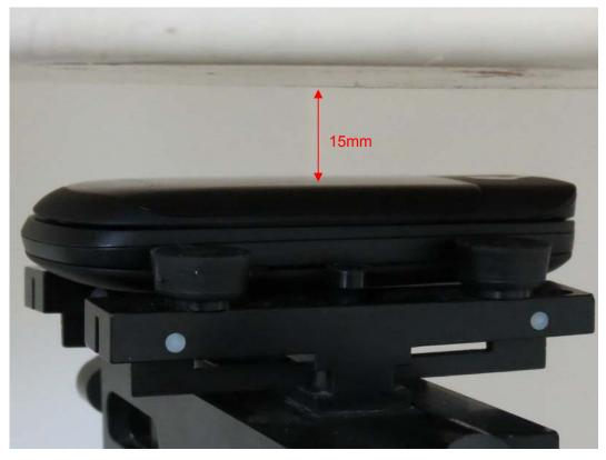
Picture 13: Body, The EUT display towards phantom, the distance from EUT to the bottom of the Phantom is 15mm (Cover Close)
