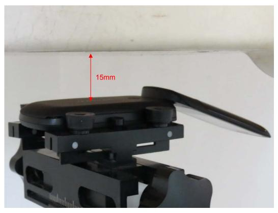
Picture 11: Body, The EUT display towards ground, the distance from EUT to the bottom of the Phantom is 15mm (Cover Open)
