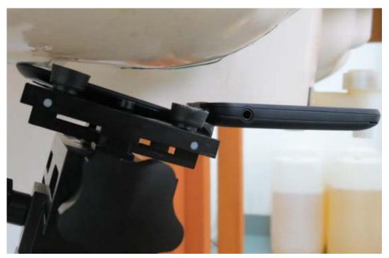
Picture 10: Right Hand Tilt 15 Degree Position (Cover Open)
