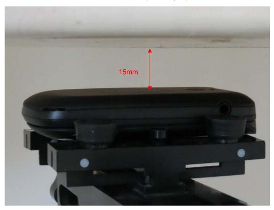
Picture 12: Body, The EUT display towards ground, the distance from EUT to the bottom of the Phantom is 15mm (Cover Close)
