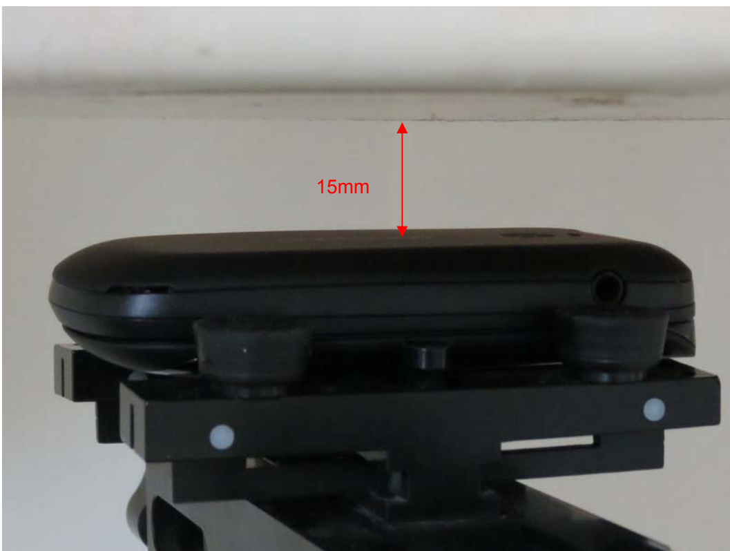
Picture 12: Body, The EUT display towards ground, the distance from EUT to the bottom of the Phantom is 15mm (Cover Close)
