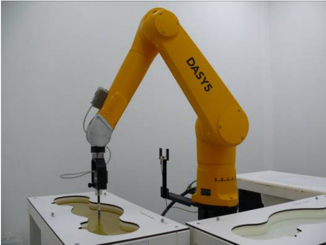
Picture 1: Specific Absorption Rate Test Layout
