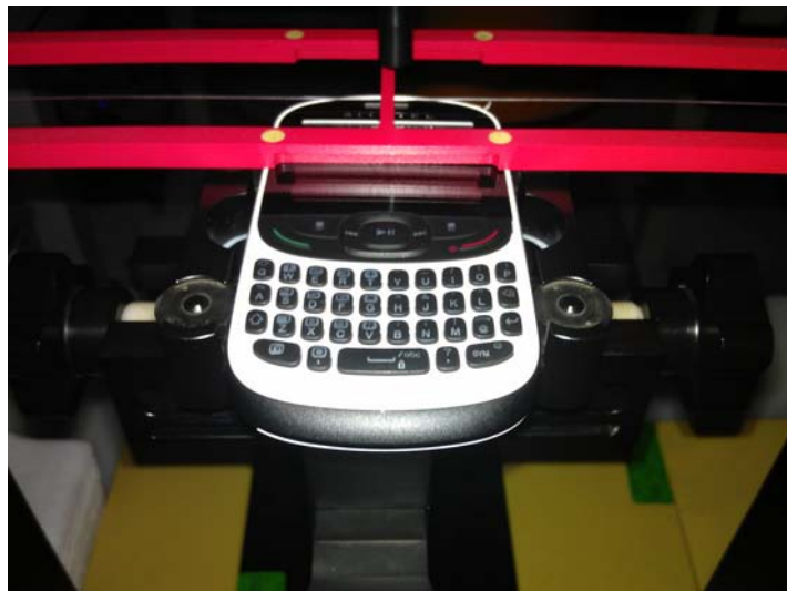
Picture 2: EUT Positioning for RF
