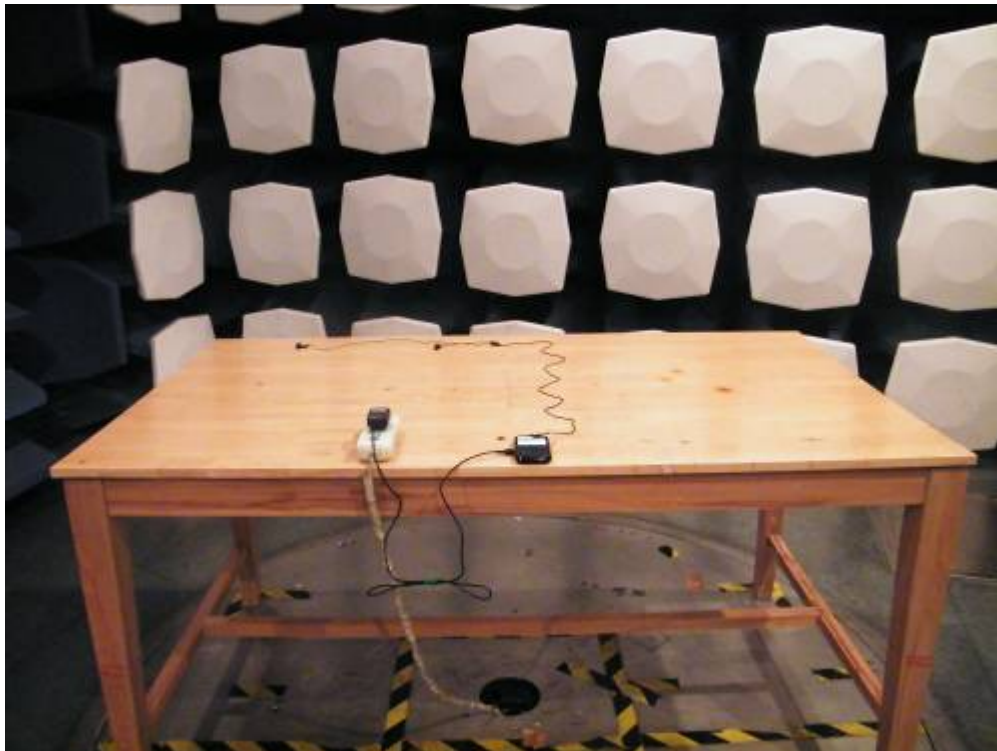
Picture 2 Radiated Emission Test Setup
