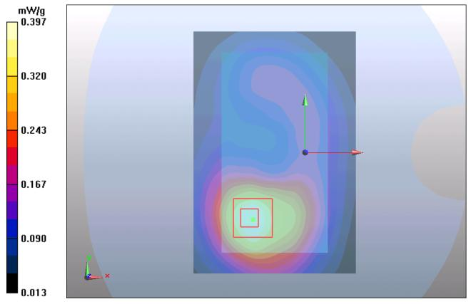
Figure 53 Body, Towards Phantom, GSM 1900 GPRS (4Txslots) Channel 512
