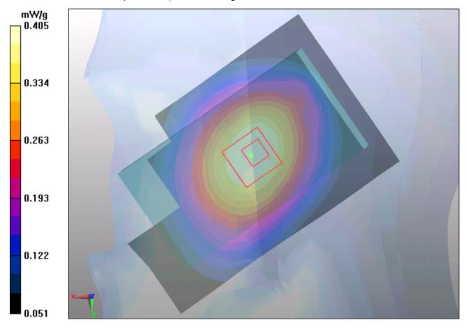
Figure 22 Right Hand Tilt 15° GSM 850 Channel 251
