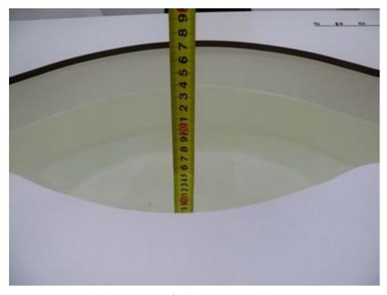
Picture 6: Liquid depth in the flat Phantom (2450 MHz, 15.4cm depth)
