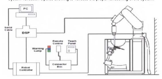
Figure 1 SAR Lab Test Measurement Set-up
