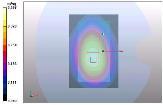
Figure 34 Body with Stereo Headset 2, Towards Ground, GSM 850 Channel 128
