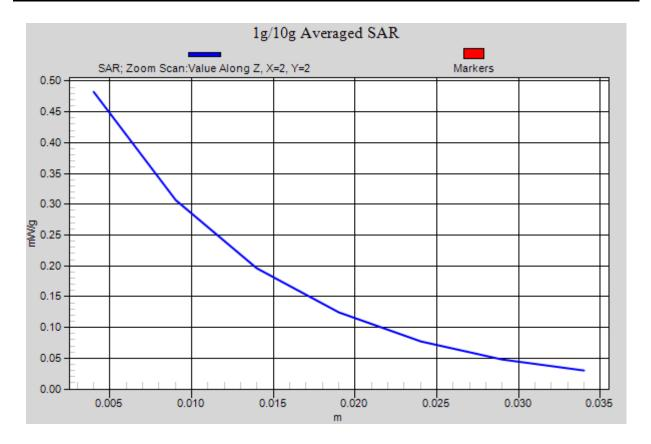
Figure 50 Body, Towards Ground, GSM 1900 GPRS (4Txslots) Channel 512
