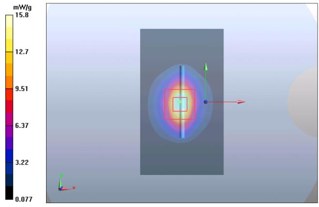
Figure 11 System Performance Check 2450MHz 250mW
