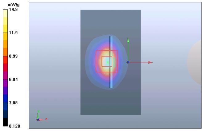
Figure 12 System Performance Check 2450MHz 250mW
