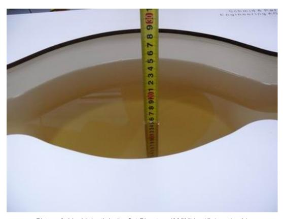
Picture 2: Liquid depth in the flat Phantom (835MHz, 15.4cm depth)
