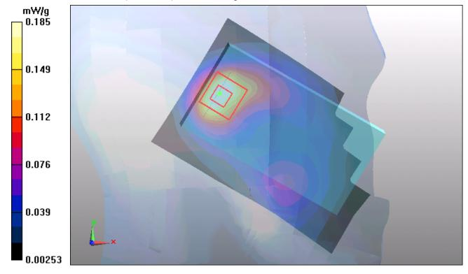
Figure 39 Left Hand Tilt 15° GSM 1900 Channel 810
