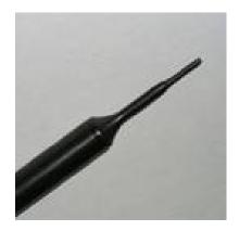
Figure 2.EX3DV4 E-field Probe
