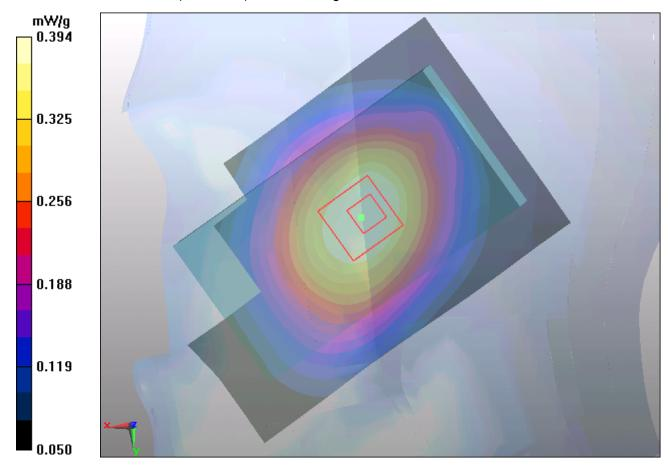
Figure 23 Right Hand Tilt 15° GSM 850 Channel 190
