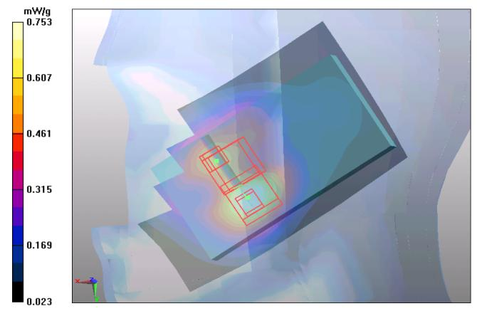
Figure 44 Right Hand Touch Cheek GSM 1900 Channel 512
