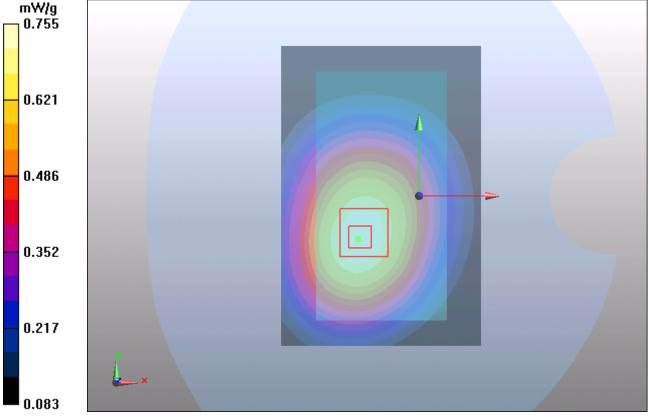
Figure 31 Body, Towards Phantom, GSM 850 GPRS (4Txslots) Channel 128
