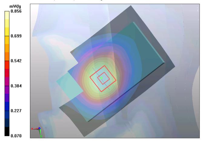
Figure 21 Right Hand Touch Cheek GSM 850 Channel 128
