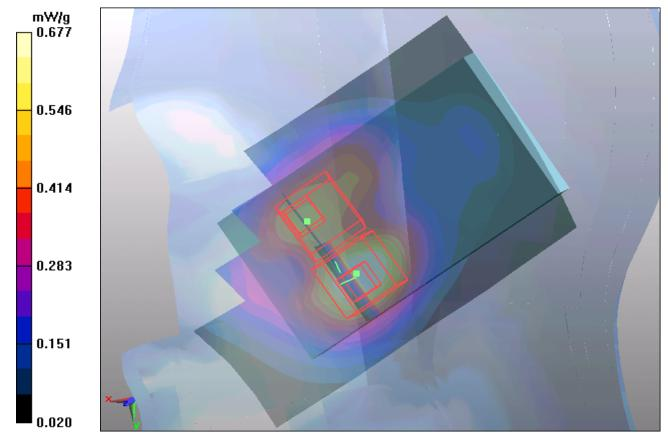
Figure 43 Right Hand Touch Cheek GSM 1900 Channel 661
