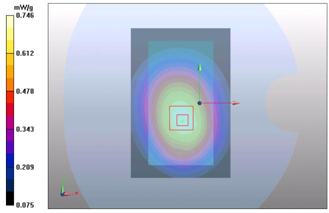
Figure 26 Body, Towards Ground, GSM 850 GPRS (4Txslots) Channel 251
