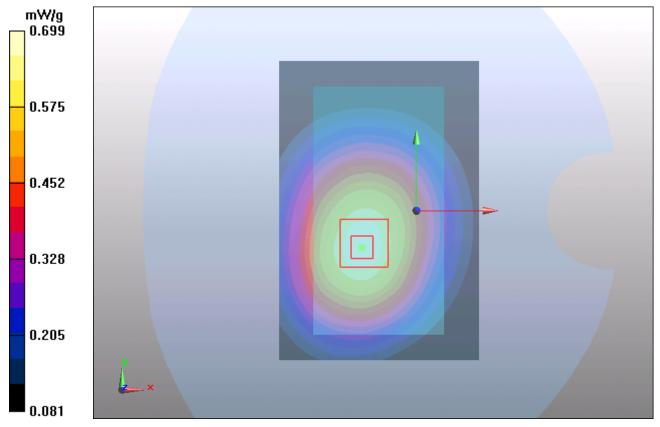
Figure 29 Body, Towards Phantom, GSM 850 GPRS (4Txslots) Channel 251
