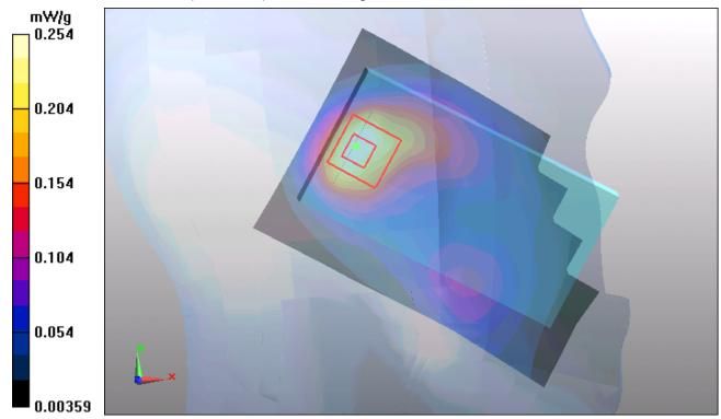
Figure 41 Left Hand Tilt 15° GSM 1900 Channel 512
