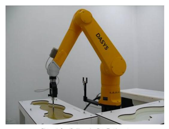
Picture 1: Specific Absorption Rate Test Layout
