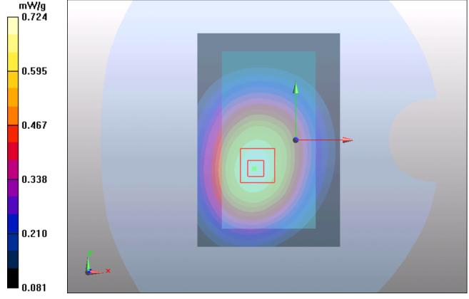
Figure 30 Body, Towards Phantom, GSM 850 GPRS (4Txslots) Channel 190
