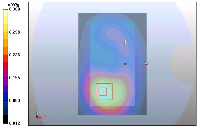
Figure 52 Body, Towards Phantom, GSM 1900 GPRS (4Txslots) Channel 661
