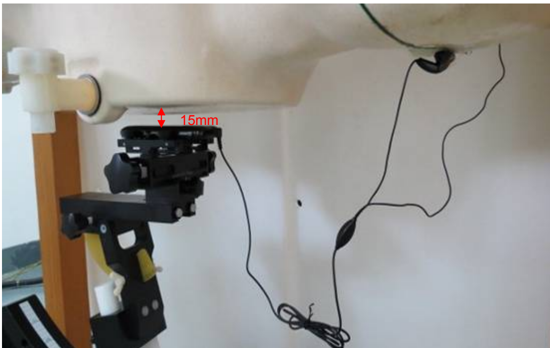
Picture 16: Body with Stereo Headset 2, The EUT display towards ground, the distance from EUT to the bottom of the Phantom is 15mm
