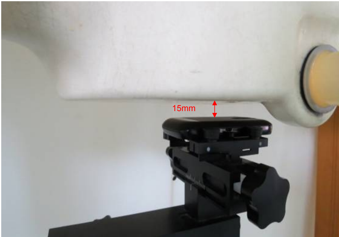
Picture 13: Body, The EUT display towards ground, the distance from EUT to the bottom of the Phantom is 15mm
