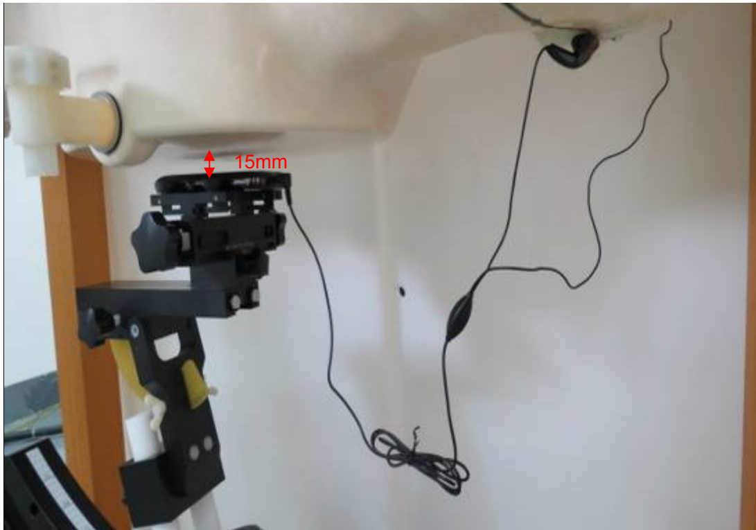
Picture 15: Body with Stereo Headset 1, The EUT display towards ground, the distance from EUT to the bottom of the Phantom is 15mm
