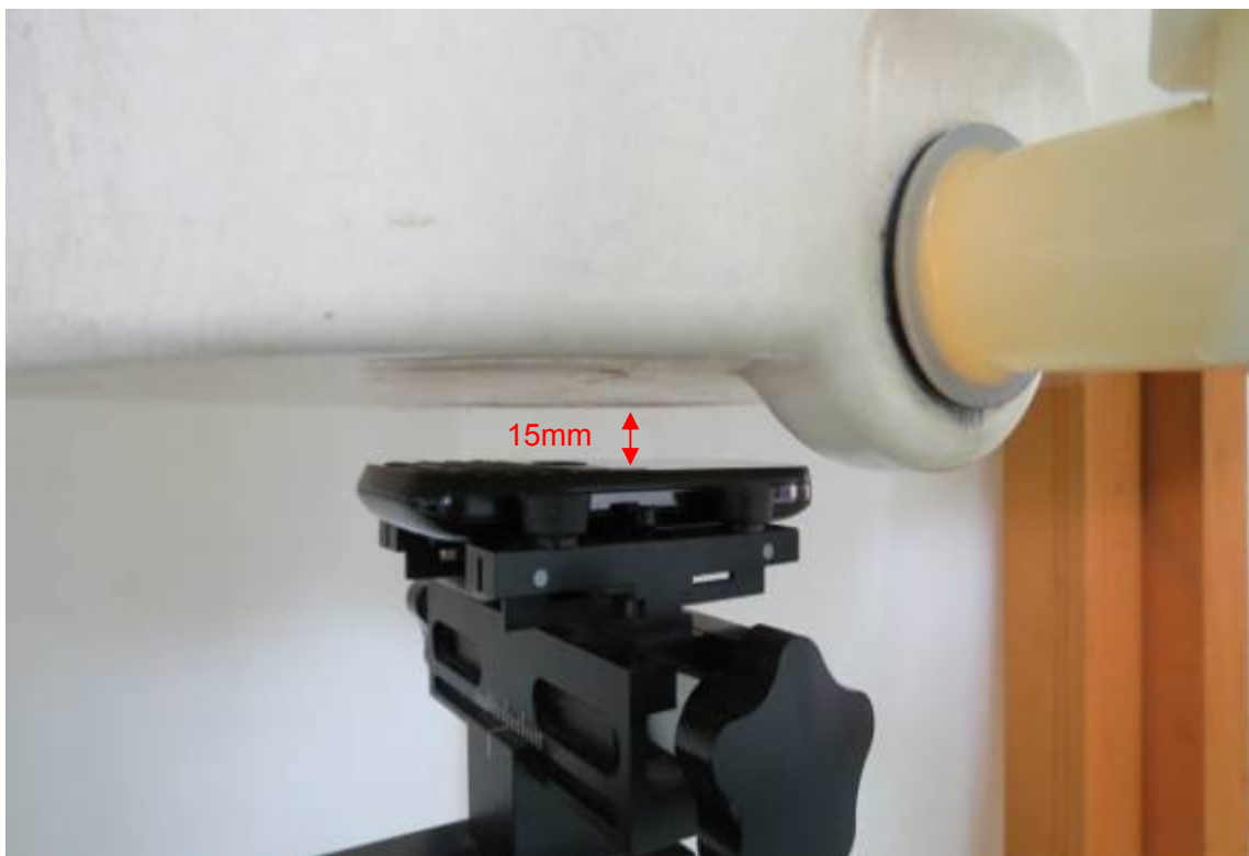
Picture 14: Body, The EUT display towards phantom, the distance from EUT to the bottom of the Phantom is 15mm
