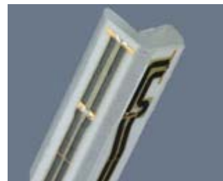
Figure 2 ER3DV6 E-field Probe
