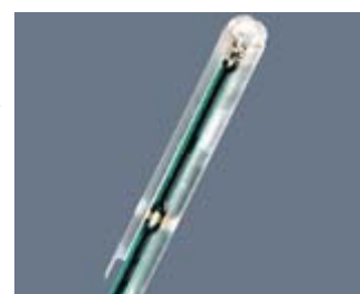
Figure 3 H3DV6 H-field Probe
