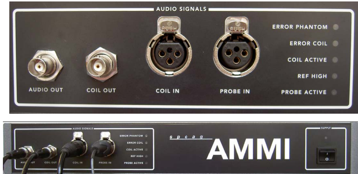
Figure 4 AMMI front panel
