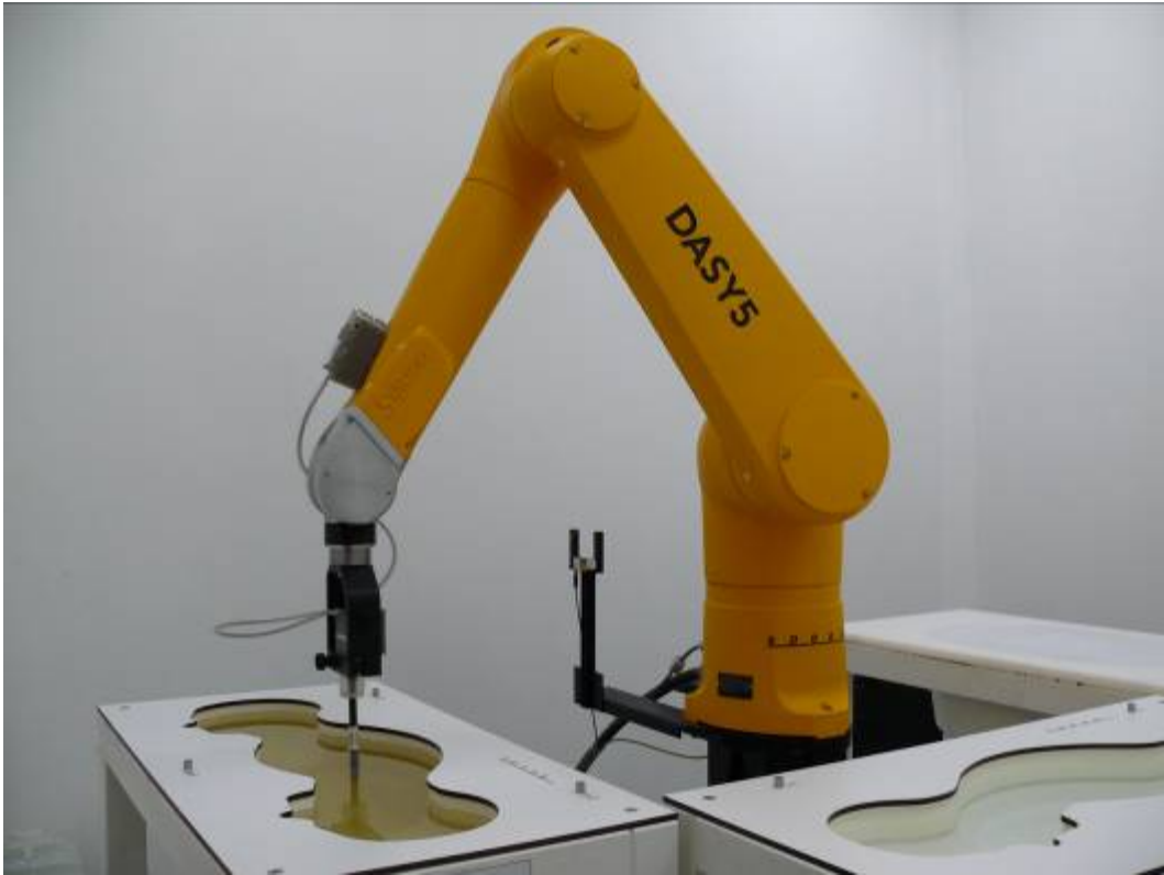
Picture 1: Specific Absorption Rate Test Layout
