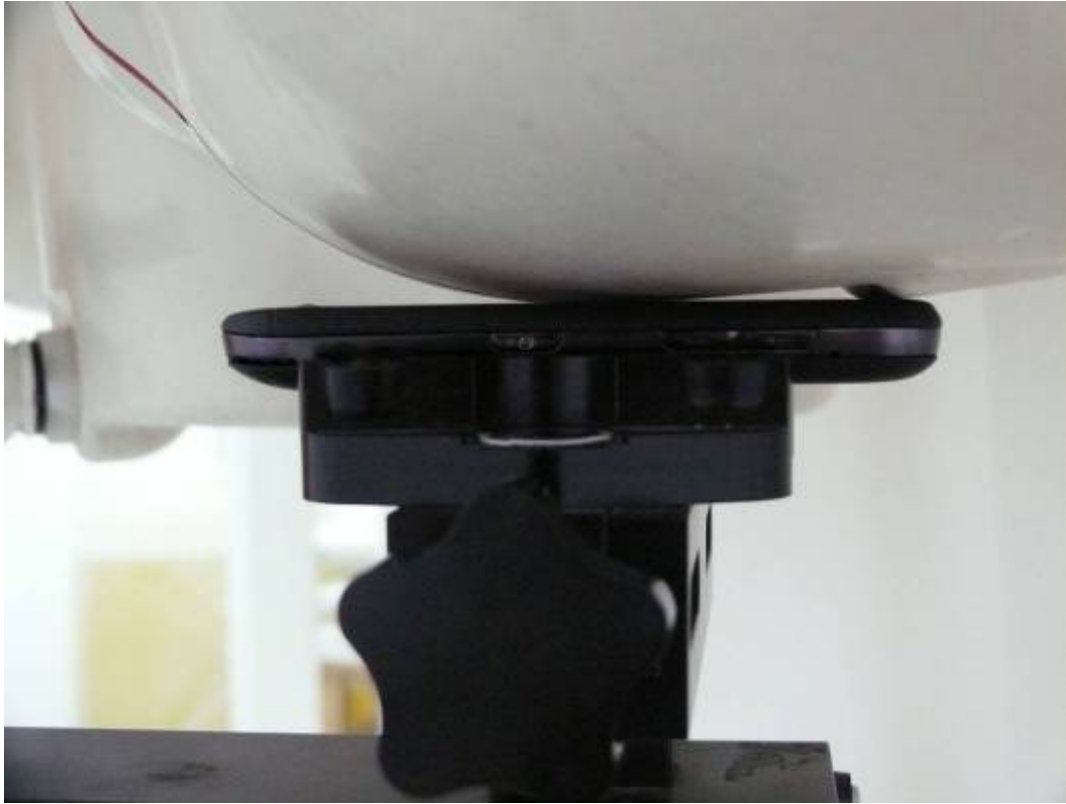
Picture 11: Left Hand Touch Cheek Position (Battery 1)
