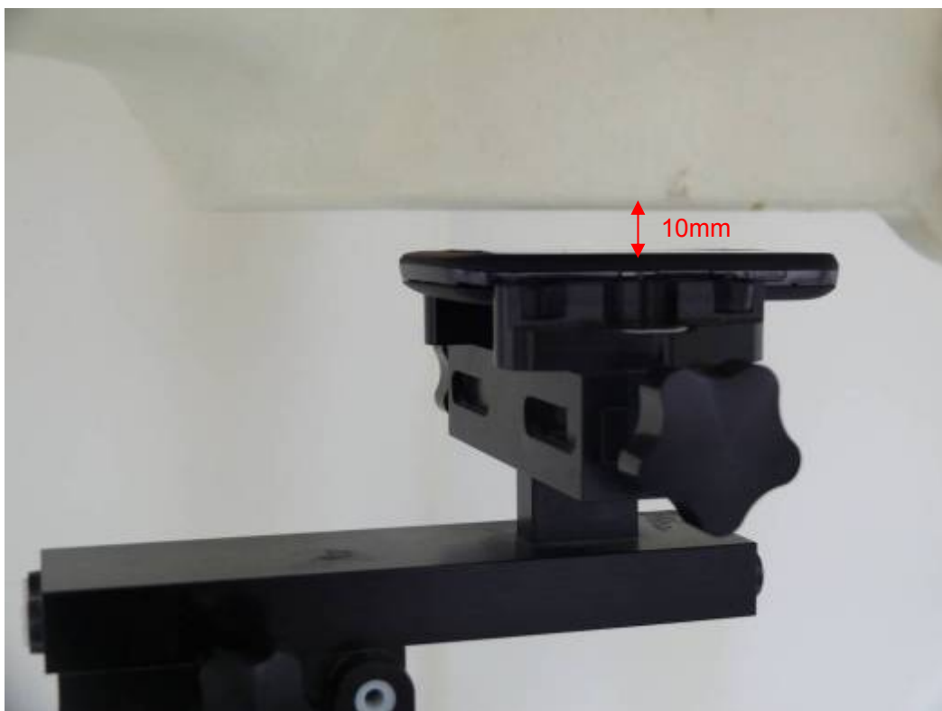
Picture 18: Front Side, the distance from handset to the bottom of the Phantom is 10mm (Battery 1)
