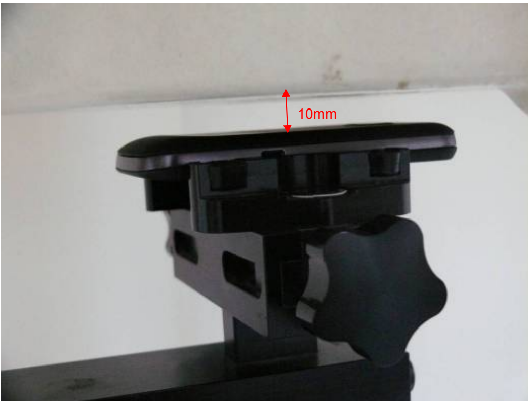
Picture 16: Back Side, the distance from handset to the bottom of the Phantom is 10mm (Battery 1)
