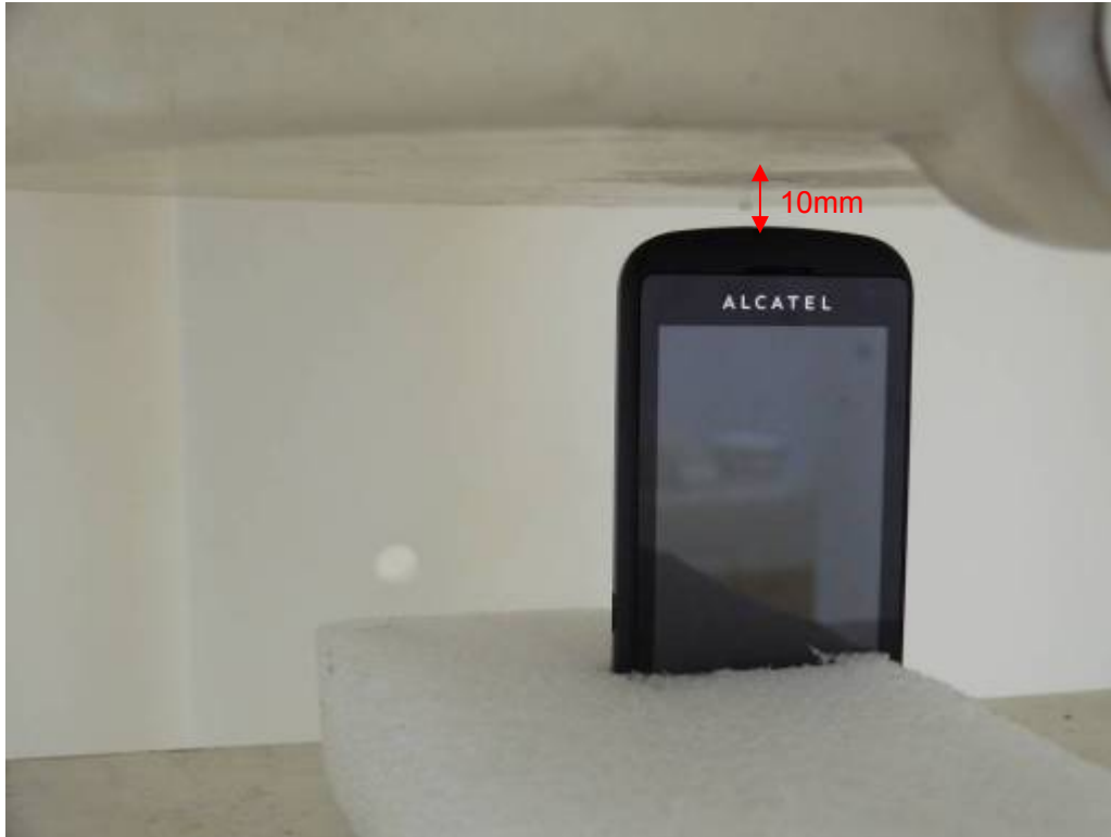
Picture 21: Top Edge, the distance from handset to the bottom of the Phantom is 10mm(Battery 1)
