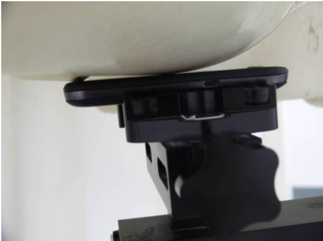
Picture 14: Right Hand Touch Cheek Position (Battery 1)
