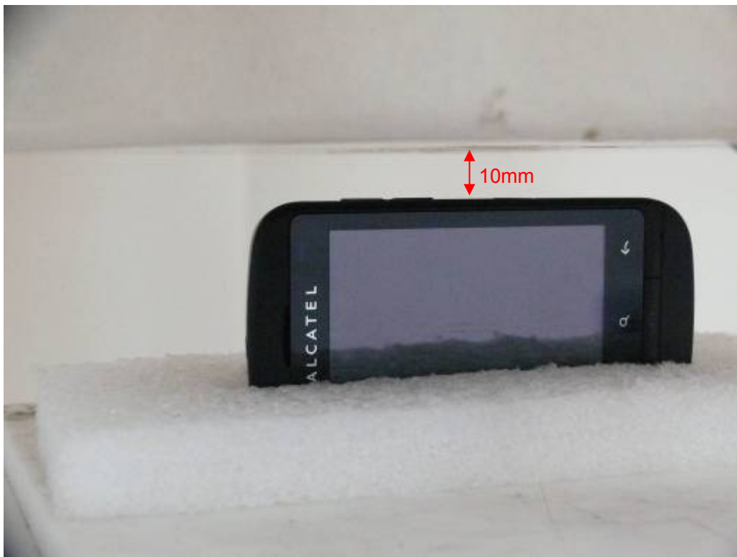
Picture 20: Right Edge, the distance from handset to the bottom of the Phantom is 10mm(Battery 1)
