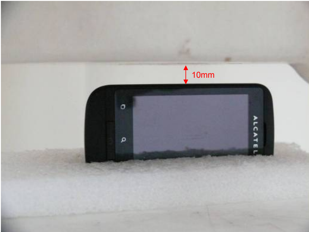
Picture 19: Left Edge, the distance from handset to the bottom of the Phantom is 10mm(Battery 1)
