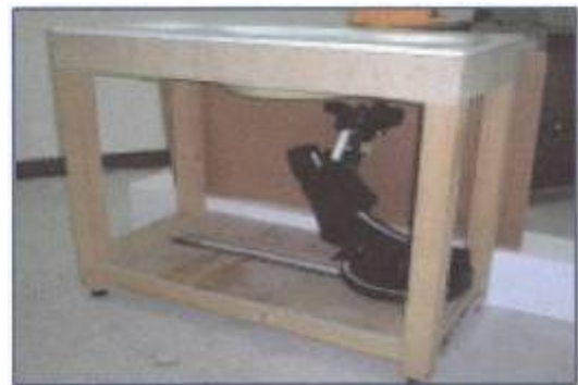
Figure 5 Generic Twin Phantom
