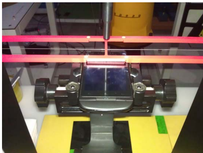
Picture 3: EUT Positioning for T-coil
