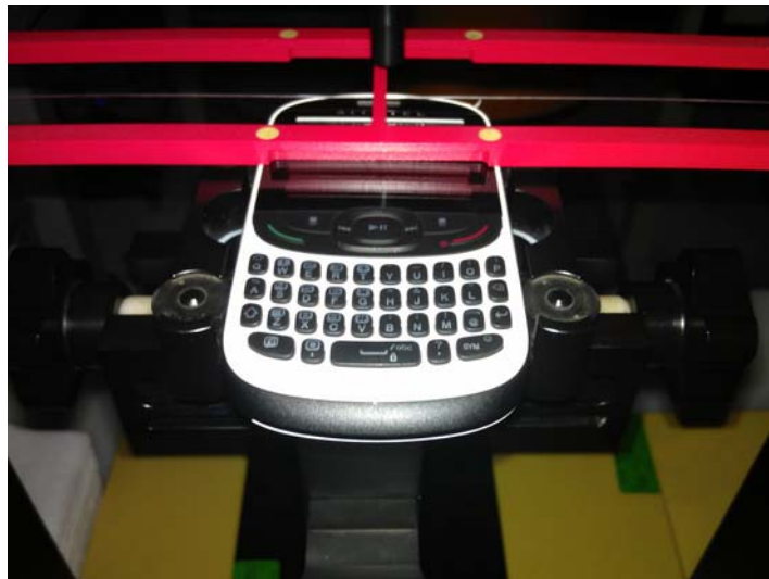
Picture 2: EUT Positioning for RF
