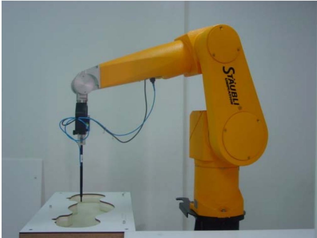
Picture 16-1: Specific Absorption Rate Test Layout
