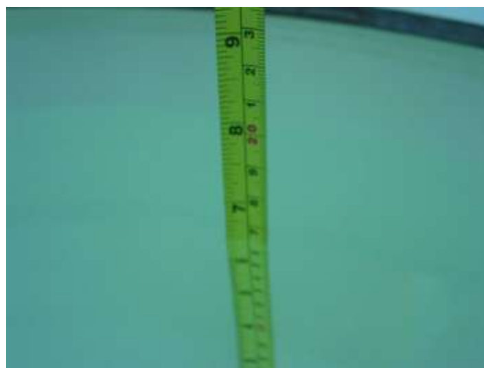
Picture 9.3 Liquid depth in the Flat Phantom (2450MHz)
