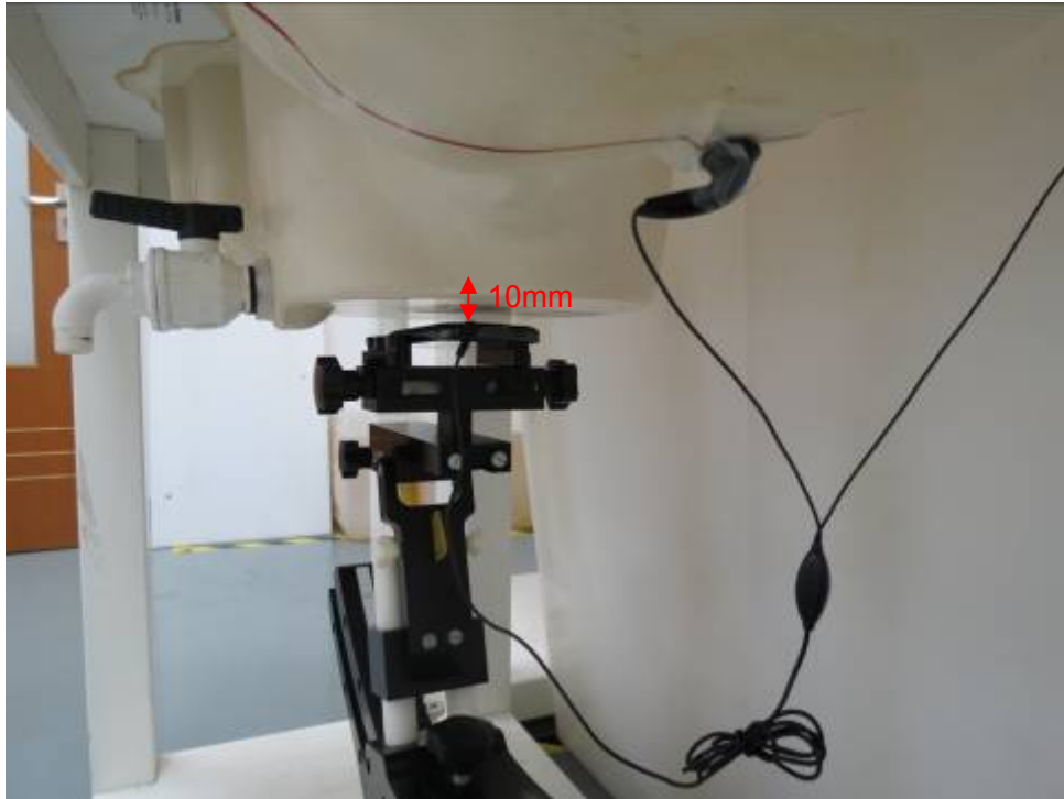
Picture 23: Back Side with Stereo Headset 1, the distance from handset to the bottom of the Phantom is 10mm (Battery 1)
