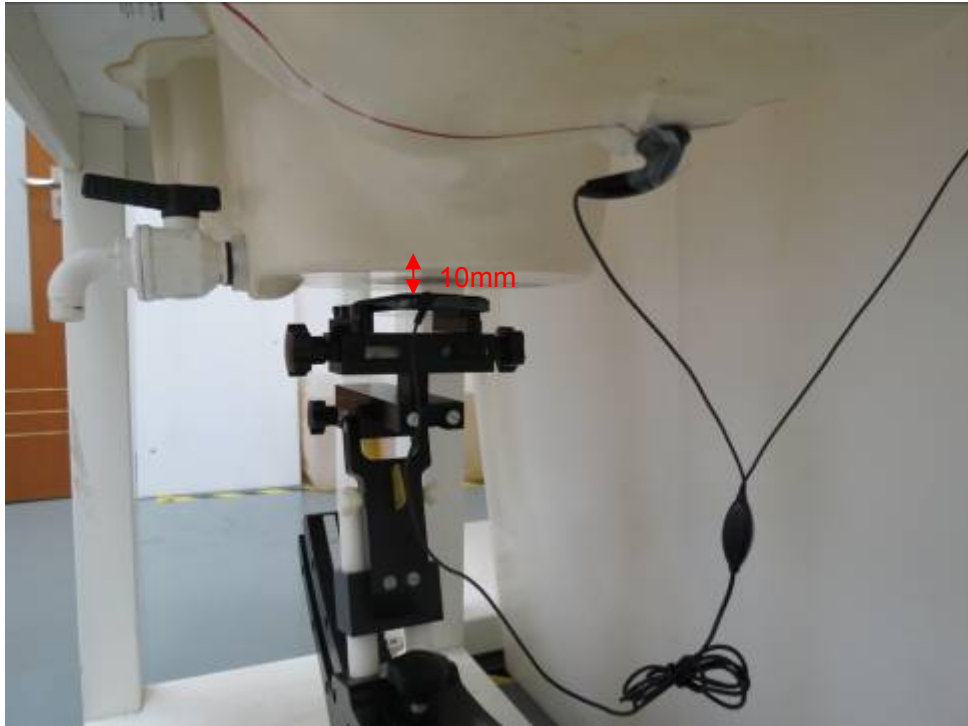
Picture 25: Back Side with Stereo Headset 3, the distance from handset to the bottom of the Phantom is 10mm (Battery 1)
