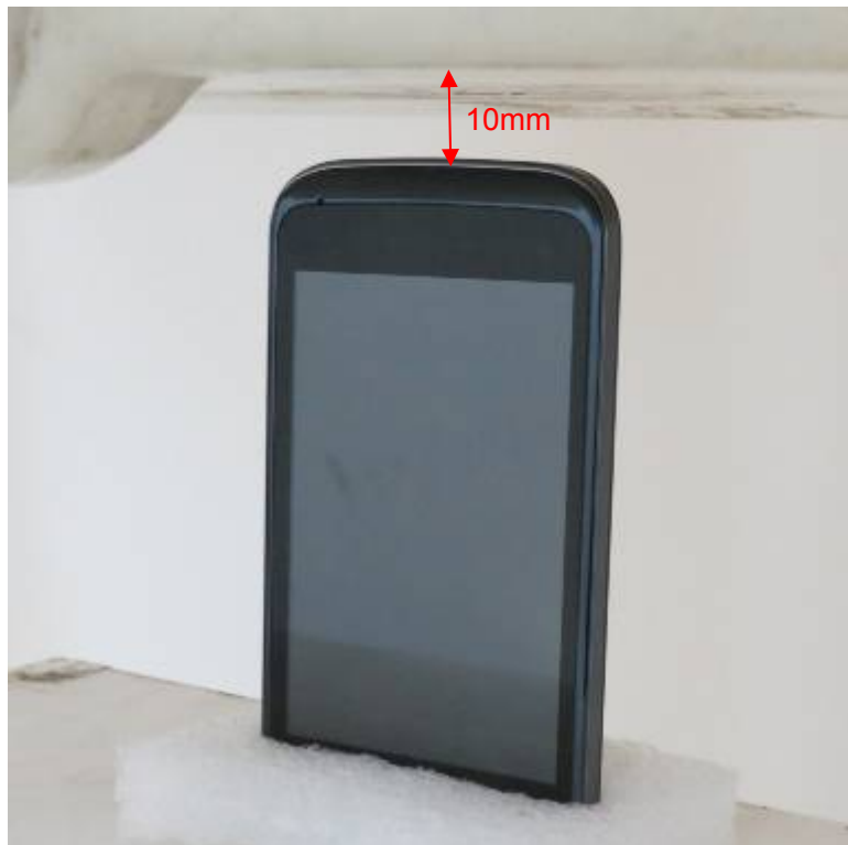
Picture 22: Bottom Edge, the distance from handset to the bottom of the Phantom is 10mm (Battery 1)
