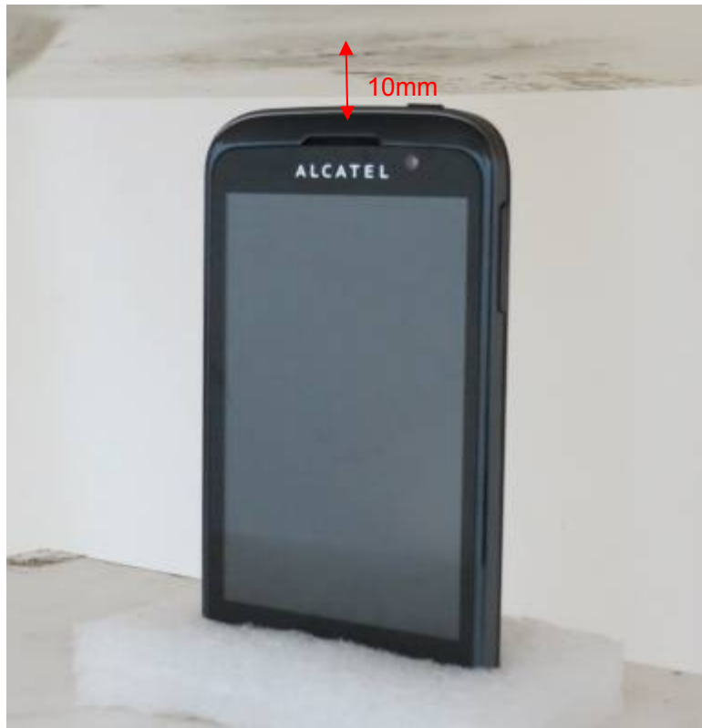
Picture 21: Top Edge, the distance from handset to the bottom of the Phantom is 10mm (Battery 1)
