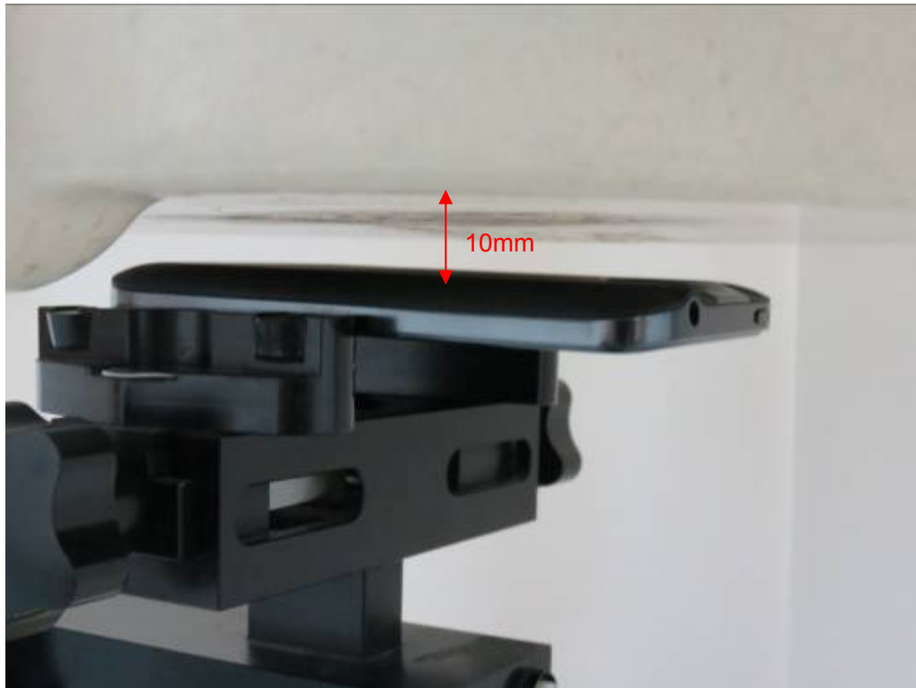
Picture 17: Back Side, the distance from handset to the bottom of the Phantom is 10mm (Battery 2)
