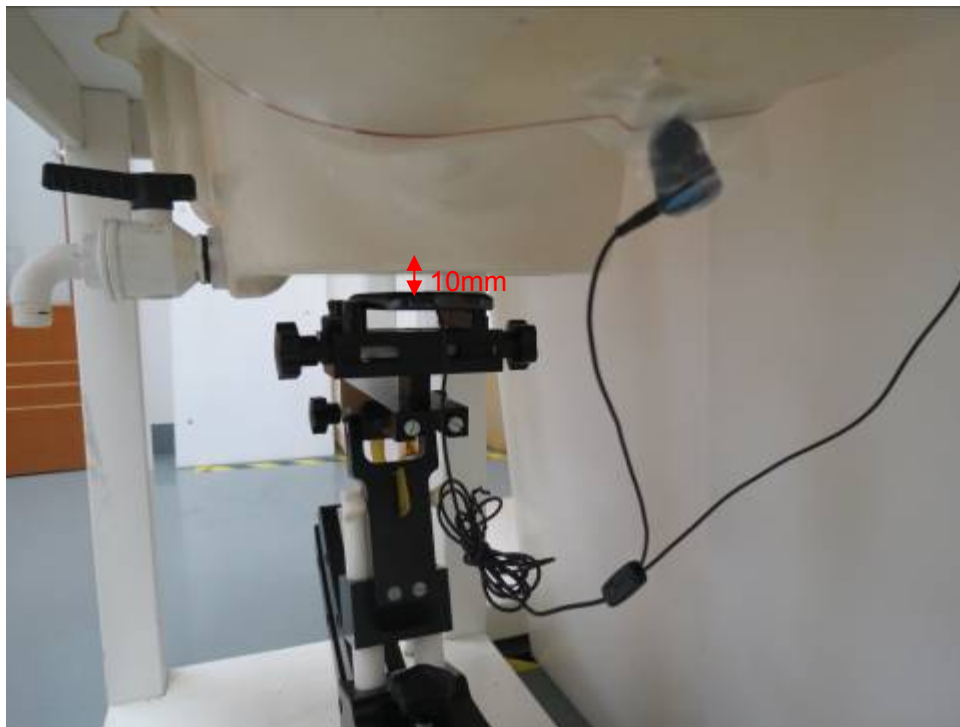
Picture 24: Back Side with Stereo Headset 2, the distance from handset to the bottom of the Phantom is 10mm (Battery 1)
