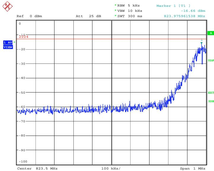
HIGH BAND EDGE BLOCK-C (GSM850) –Channel 251
