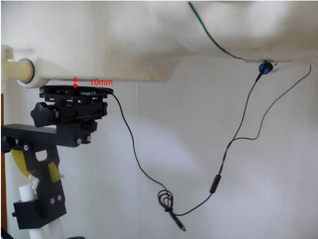
Picture 23: Back Side with Stereo Headset 3, the distance from handset to the bottom of the Phantom is 10mm (Battery 1)
