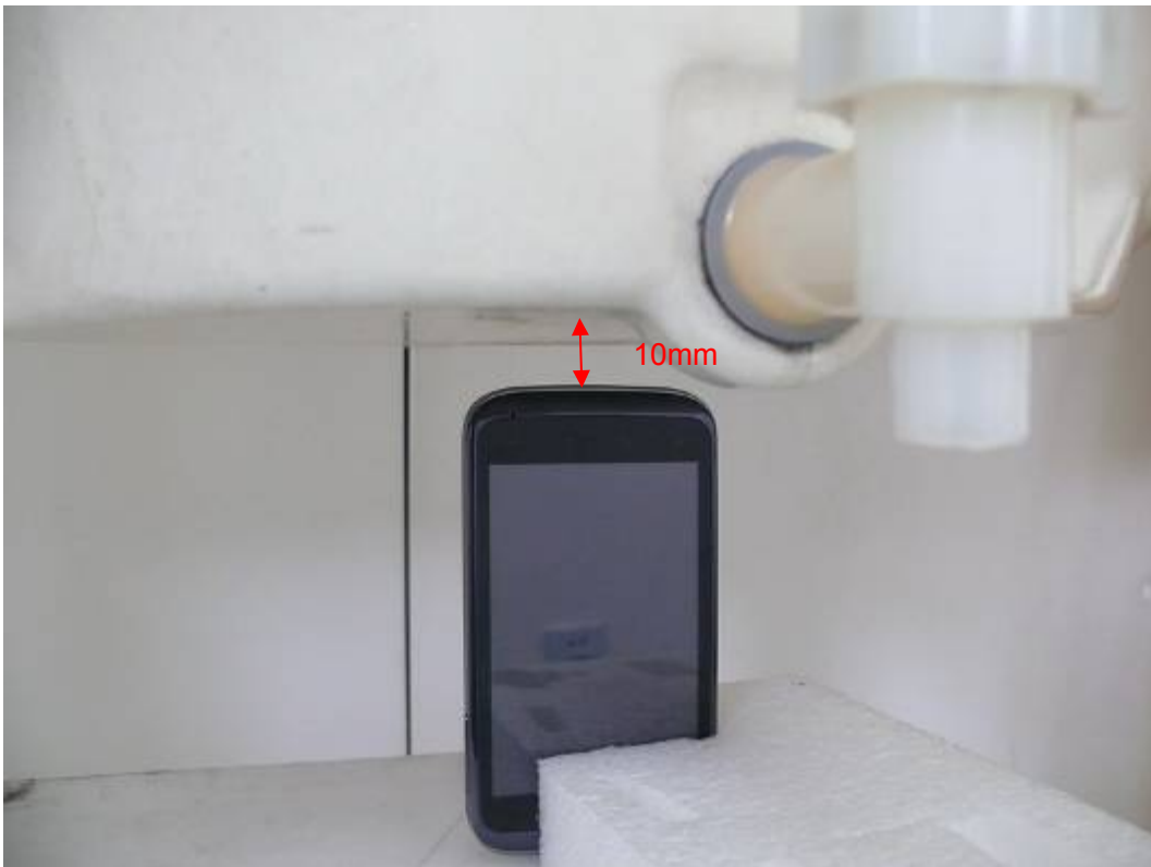
Picture 19: Bottom Edge, the distance from handset to the bottom of the Phantom is 10mm (Battery 1)
