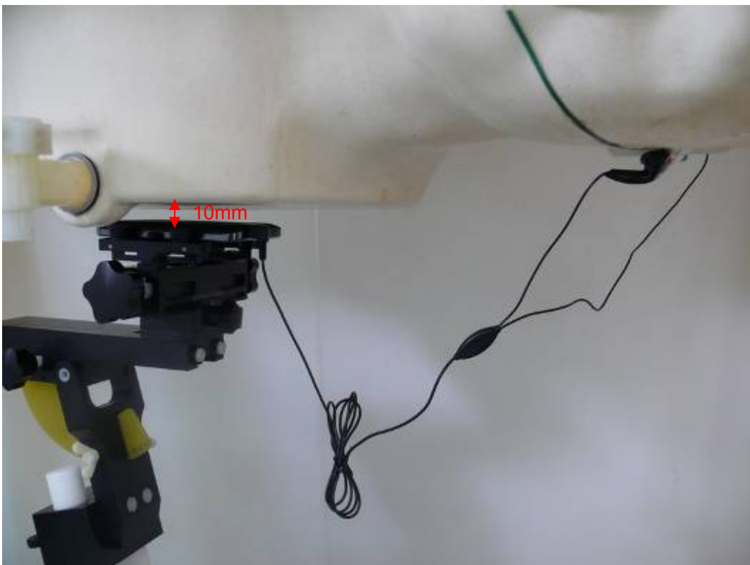
Picture 22: Back Side with Stereo Headset 2, the distance from handset to the bottom of the Phantom is 10mm (Battery 1)
