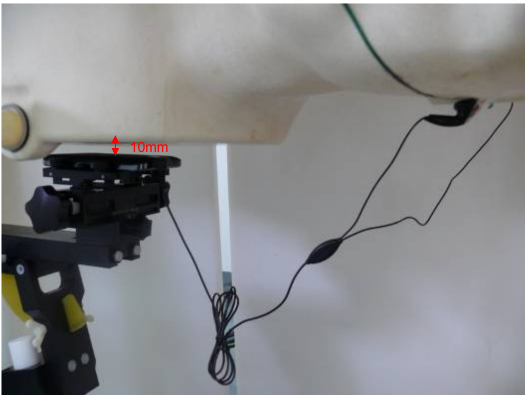
Picture 20: Back Side with Stereo Headset 1, the distance from handset to the bottom of the Phantom is 10mm (Battery 1)
