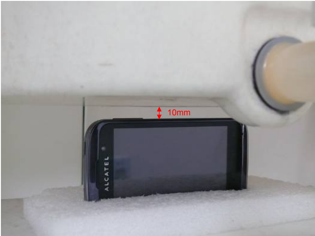
Picture 17: Right Edge, the distance from handset to the bottom of the Phantom is 10mm (Battery 1)
