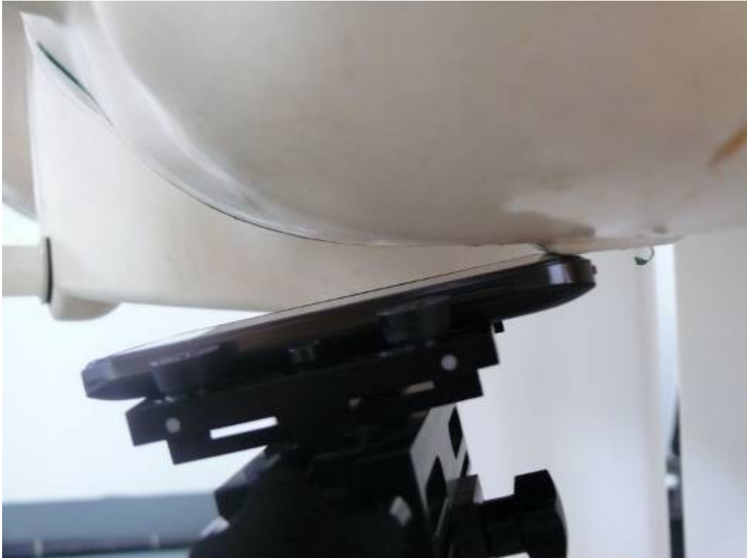
Picture 11: Left Hand Tilt 15 Degree Position (Battery 1)
