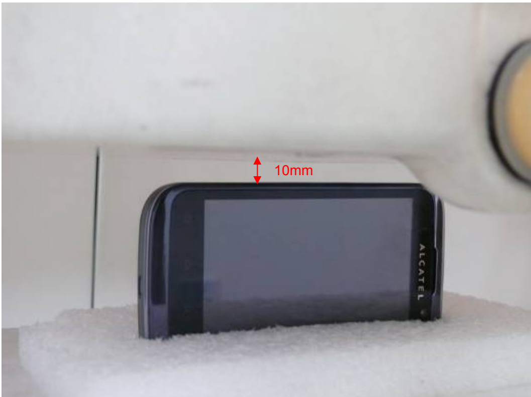
Picture 16: Left Edge, the distance from handset to the bottom of the Phantom is 10mm (Battery 1)
