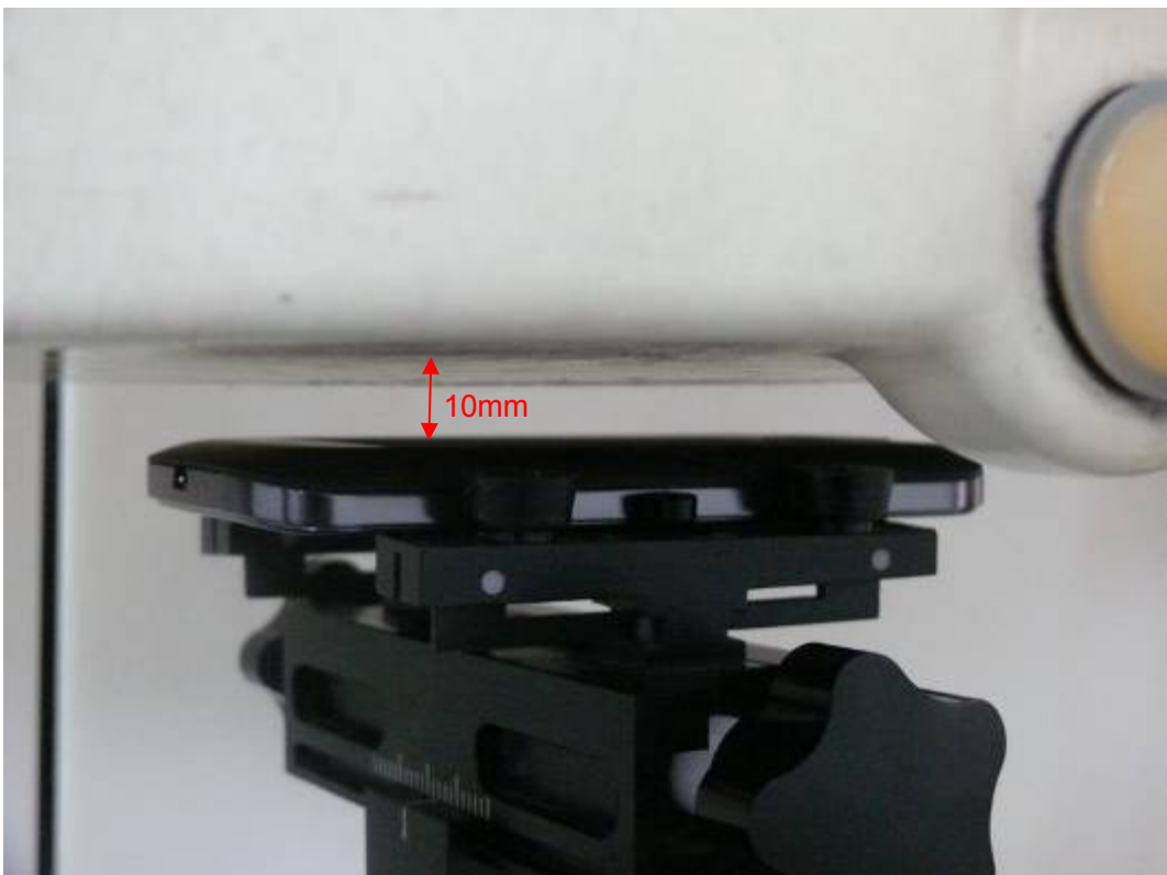
Picture 14: Back Side, the distance from handset to the bottom of the Phantom is 10mm (Battery 1)
