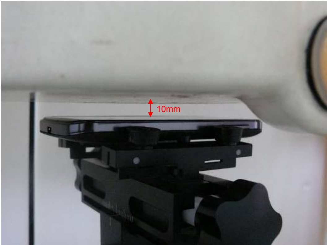
Picture 15: Front Side, the distance from handset to the bottom of the Phantom is 10mm (Battery 1)
