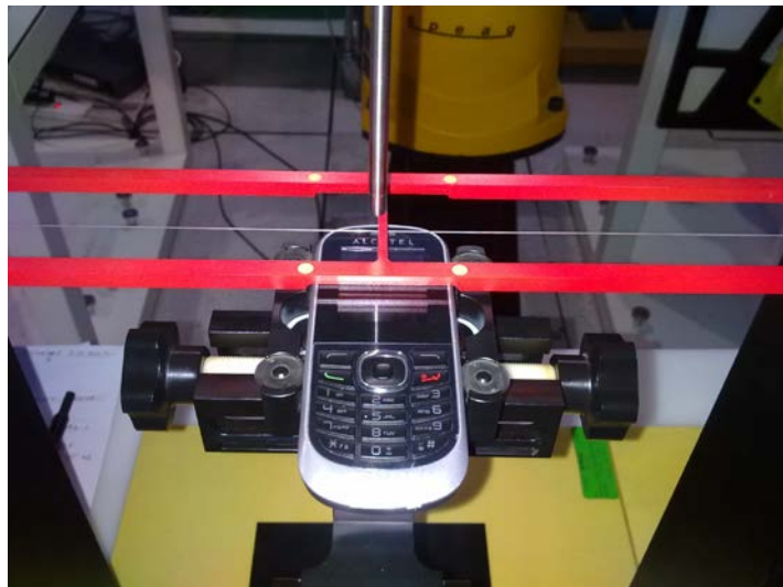
Picture 3: EUT Positioning for T-coil
