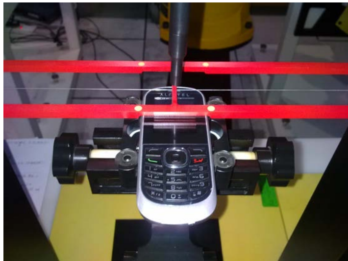
Picture 2: EUT Positioning for RF
