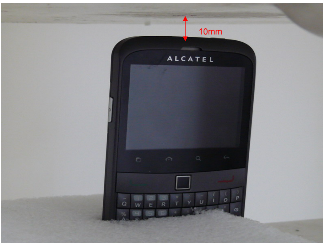
Picture 18: Top Edge, the distance from handset to the bottom of the Phantom is 10mm (Battery 1)
