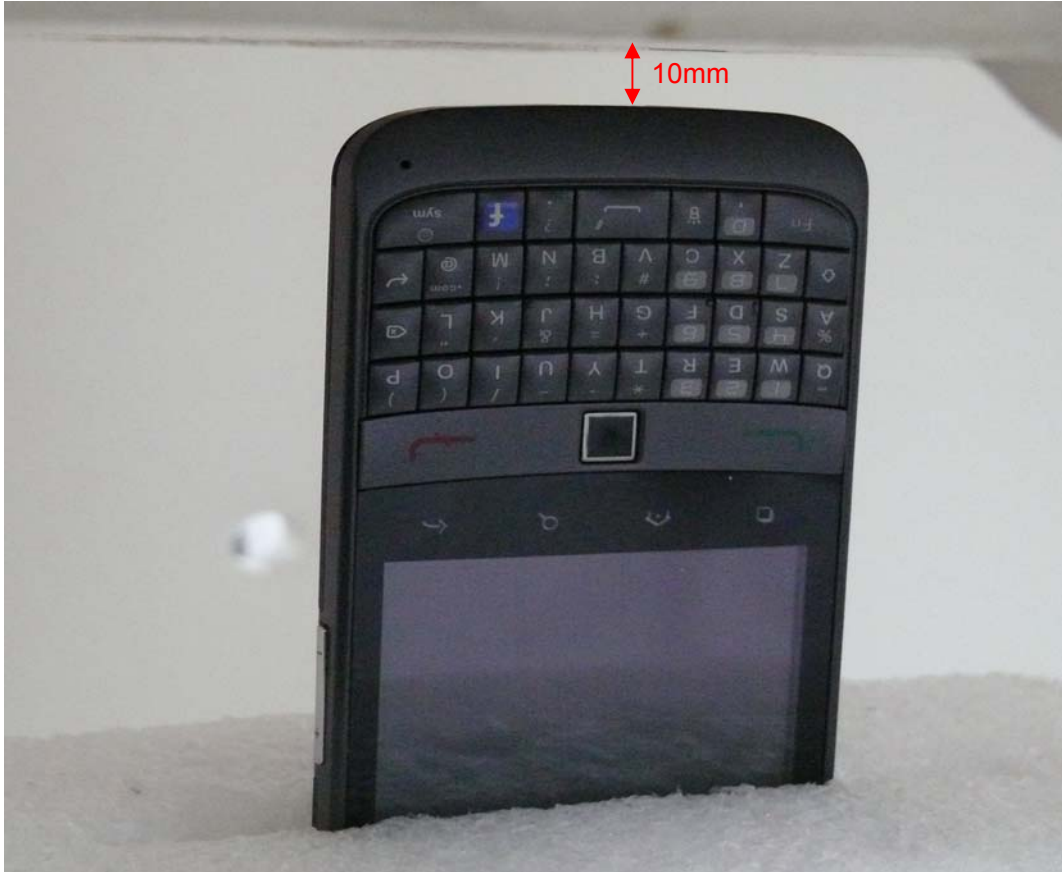
Picture 19: Bottom Edge, the distance from handset to the bottom of the Phantom is 10mm (Battery 1)
