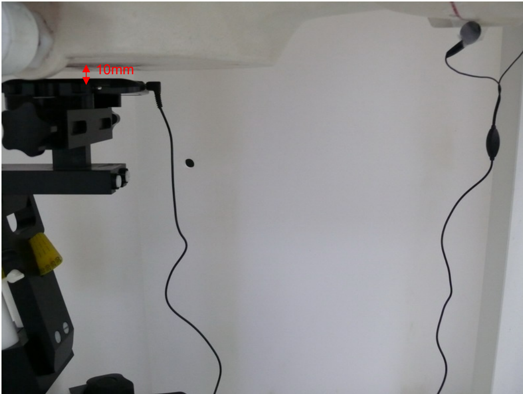
Picture 21: Back Side with Stereo Headset 2, the distance from handset to the bottom of the Phantom is 10mm (Battery 1)
