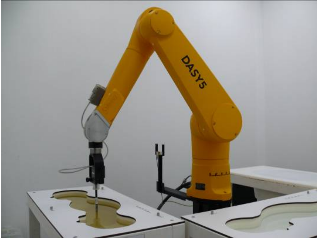
Picture 1: Specific Absorption Rate Test Layout
