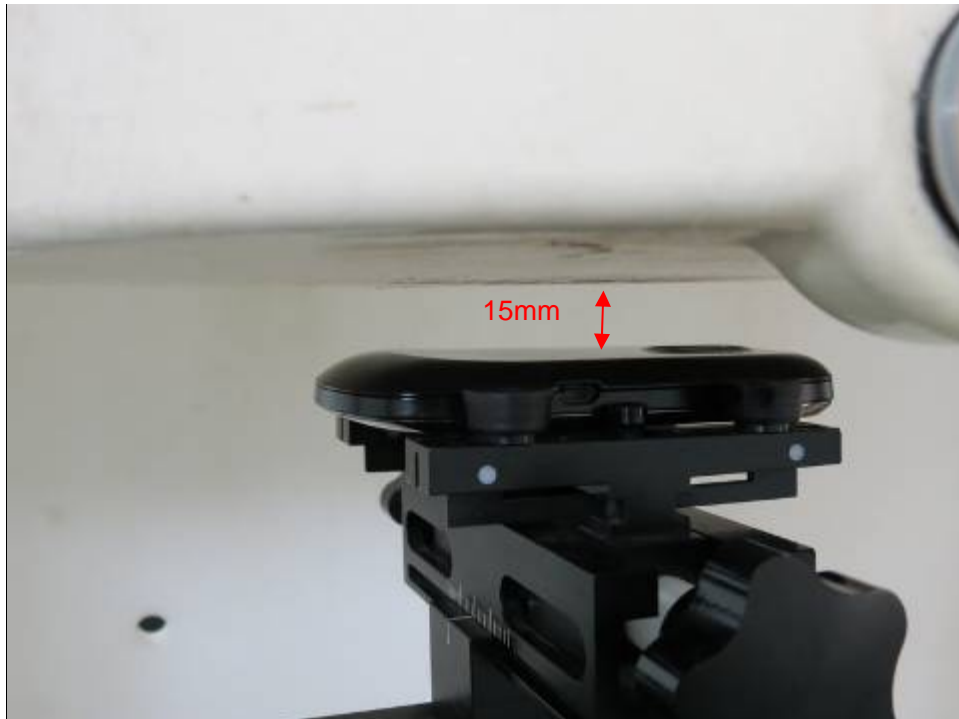
Picture 15: Body, The EUT display towards ground, the distance from EUT to the bottom of the Phantom is 15mm (Battery 2)
