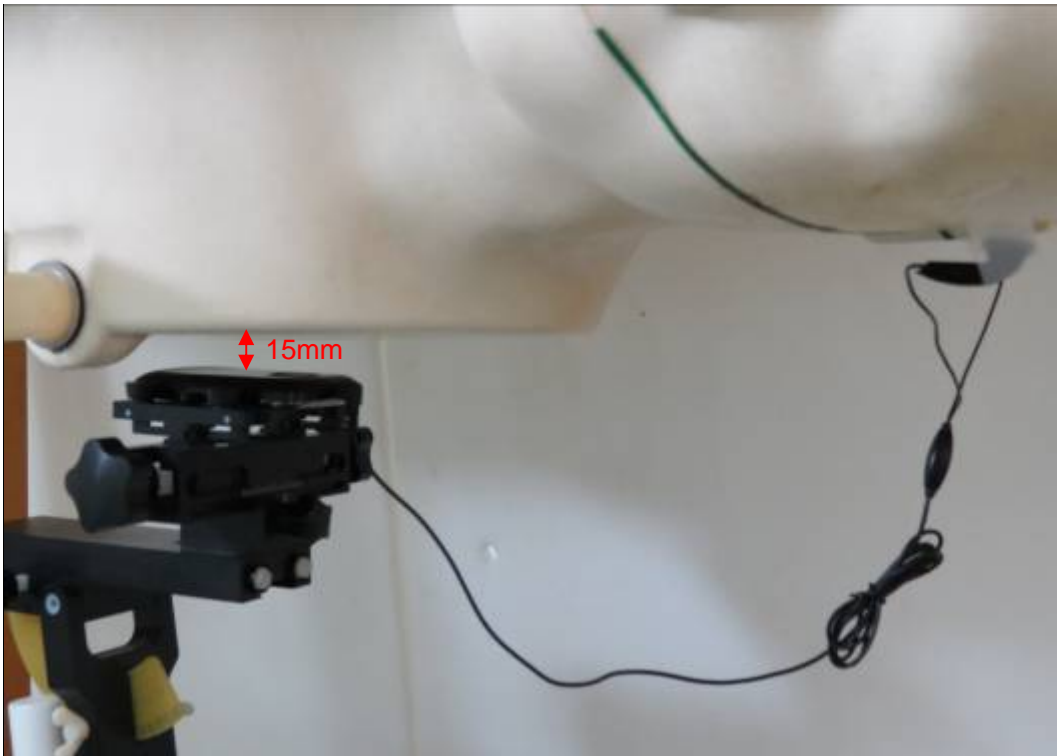
Picture 17: Body with Stereo Headset 1, The EUT display towards ground, the distance from EUT to the bottom of the Phantom is 15mm (Battery 1)
