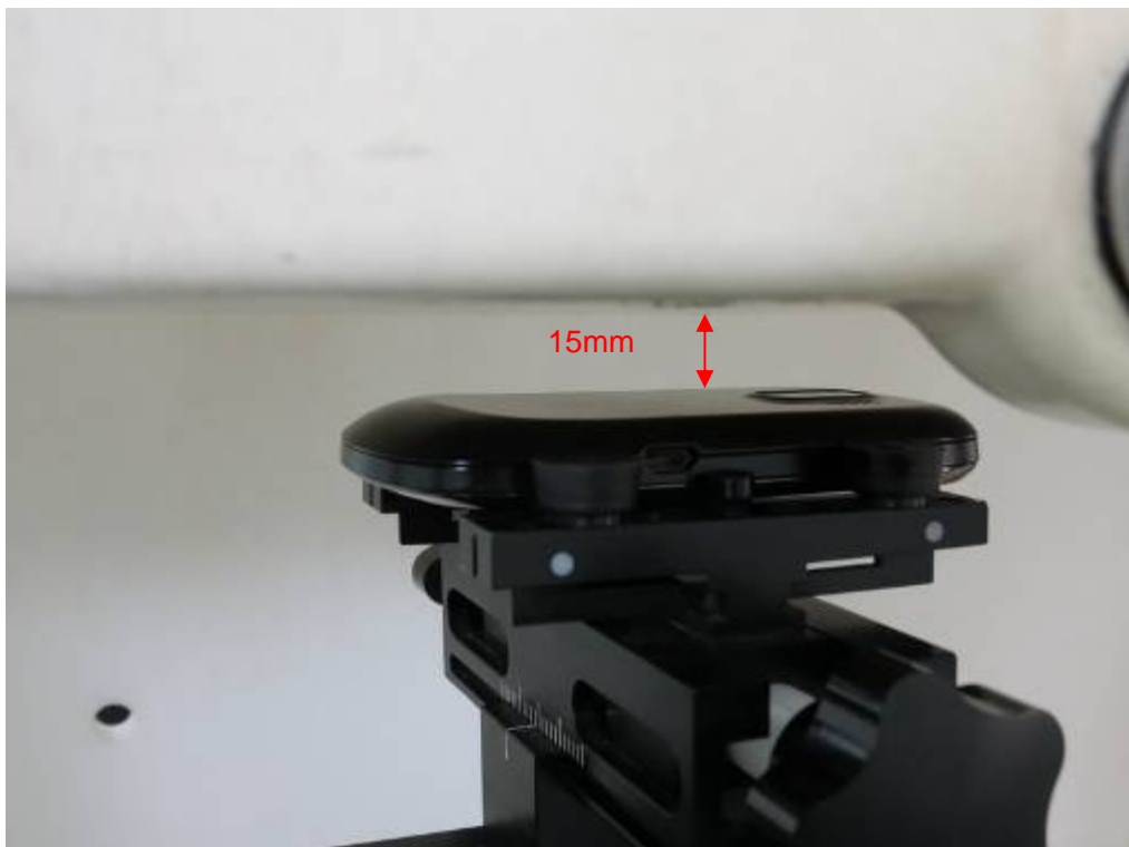
Picture 14: Body, The EUT display towards ground, the distance from EUT to the bottom of the Phantom is 15mm (Battery 1)
