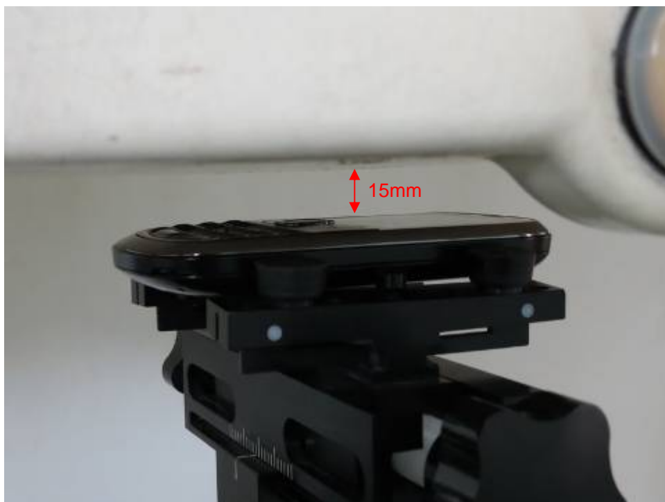
Picture 16: Body, The EUT display towards phantom, the distance from EUT to the bottom of the Phantom is 15mm (Battery 1)
