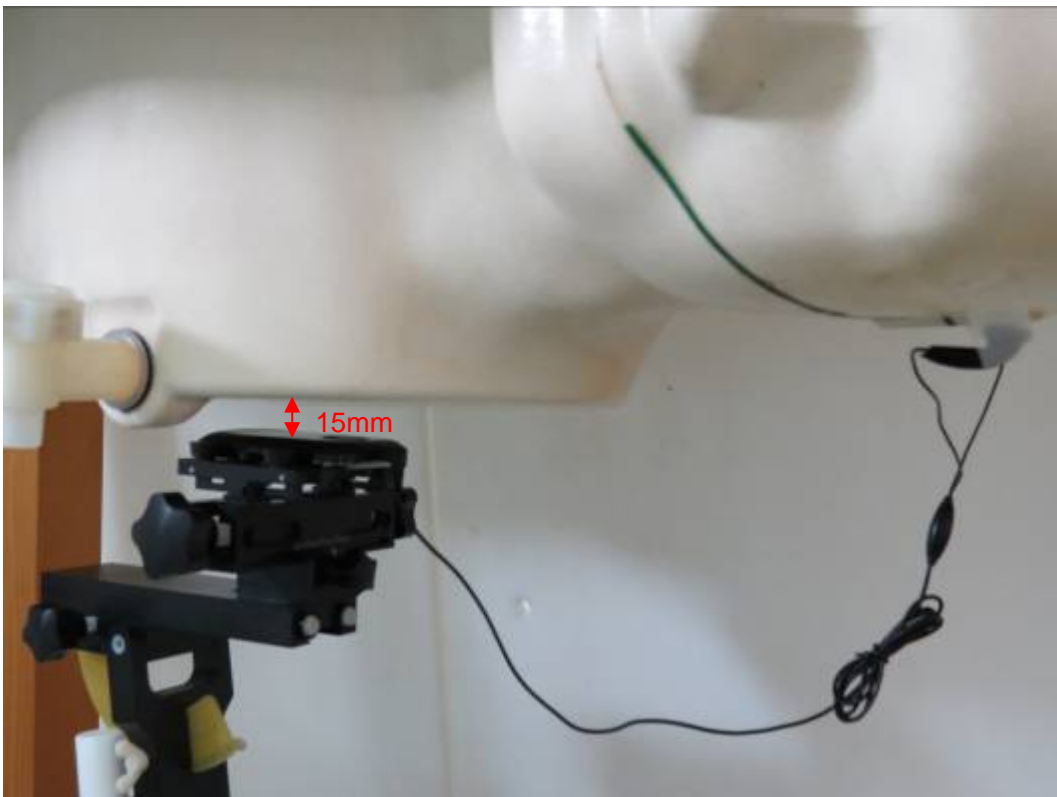
Picture 18: Body with Stereo Headset 2, The EUT display towards ground, the distance from EUT to the bottom of the Phantom is 15mm (Battery 1)
