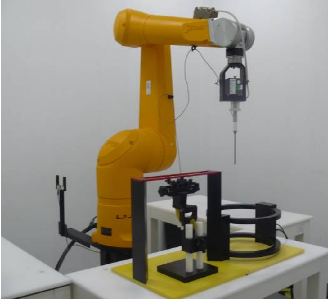
Picture 1: HAC T-Coil System Layout
