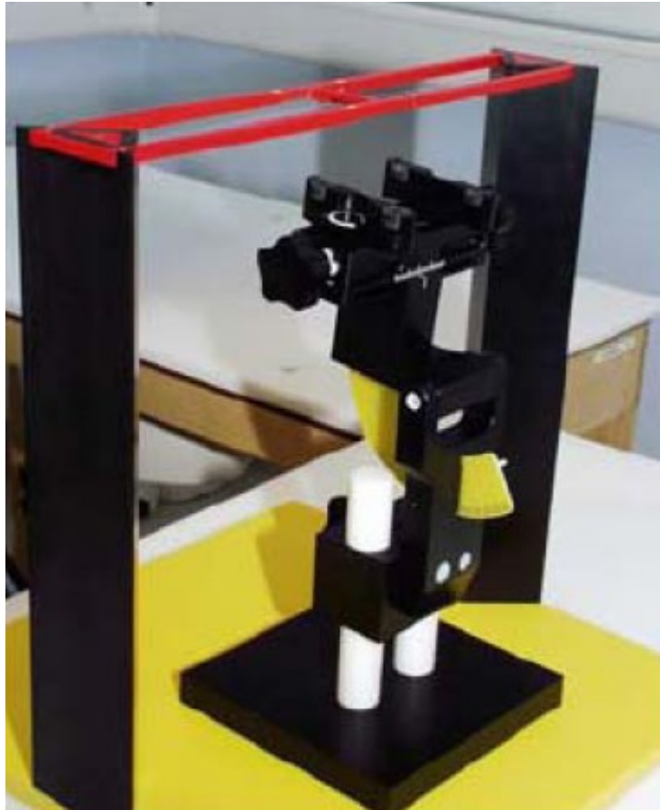
Figure 7 T-coil Phantom & Device Holder
