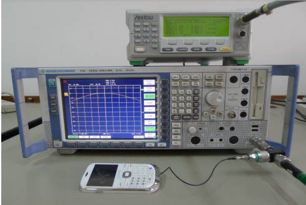
Spurious RF Conducted Emissions Test setup
