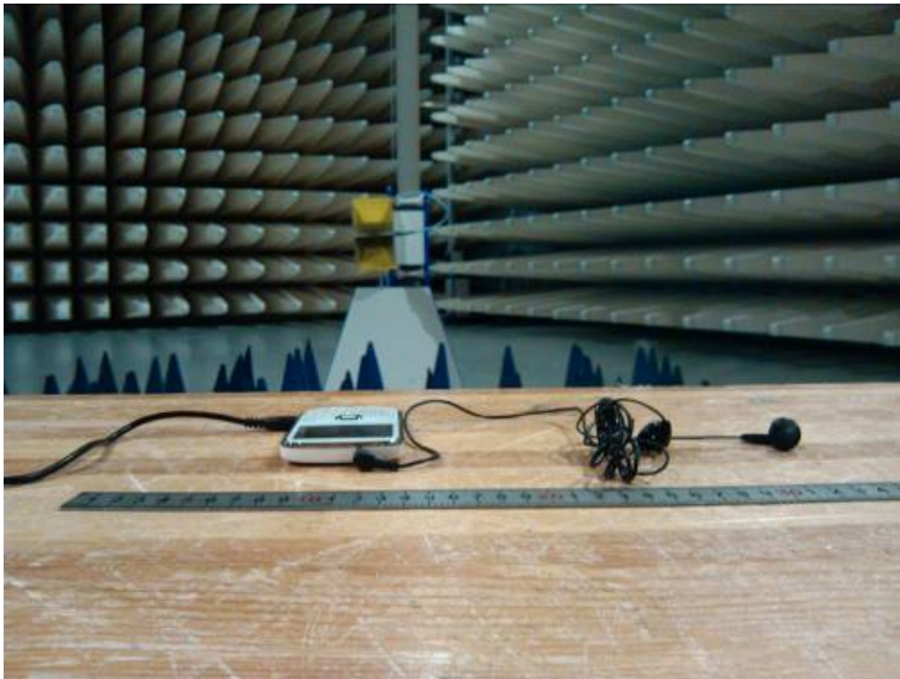
Spurious Radiated Emissions Test setup
