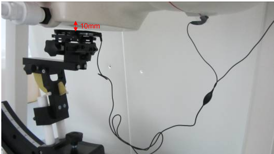
Picture 24: Back Side with Stereo Headset 2, the distance from handset to the bottom of the Phantom is 10mm (Battery 1)
