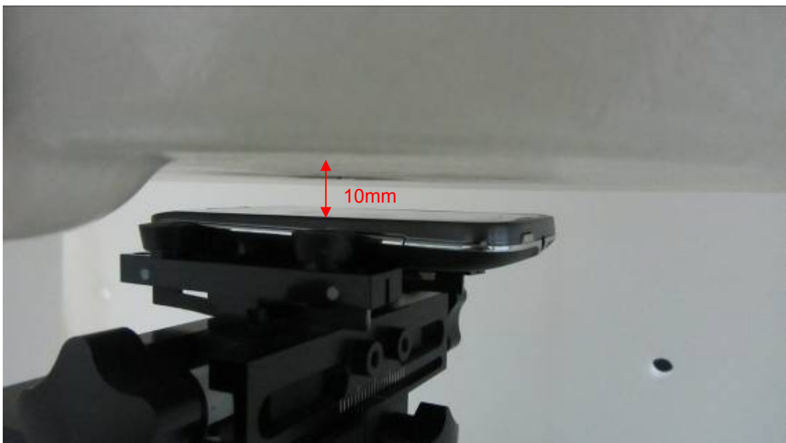
Picture 18: Front Side, the distance from handset to the bottom of the Phantom is 10mm (Battery 1)
