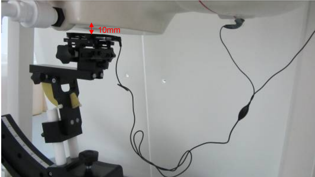
Picture 23: Back Side with Stereo Headset 1, the distance from handset to the bottom of the Phantom is 10mm (Battery 1)
