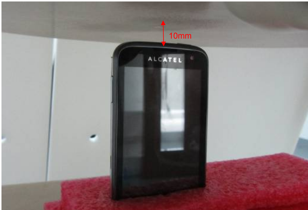
Picture 21: Top Edge, the distance from handset to the bottom of the Phantom is 10mm (Battery 1)
