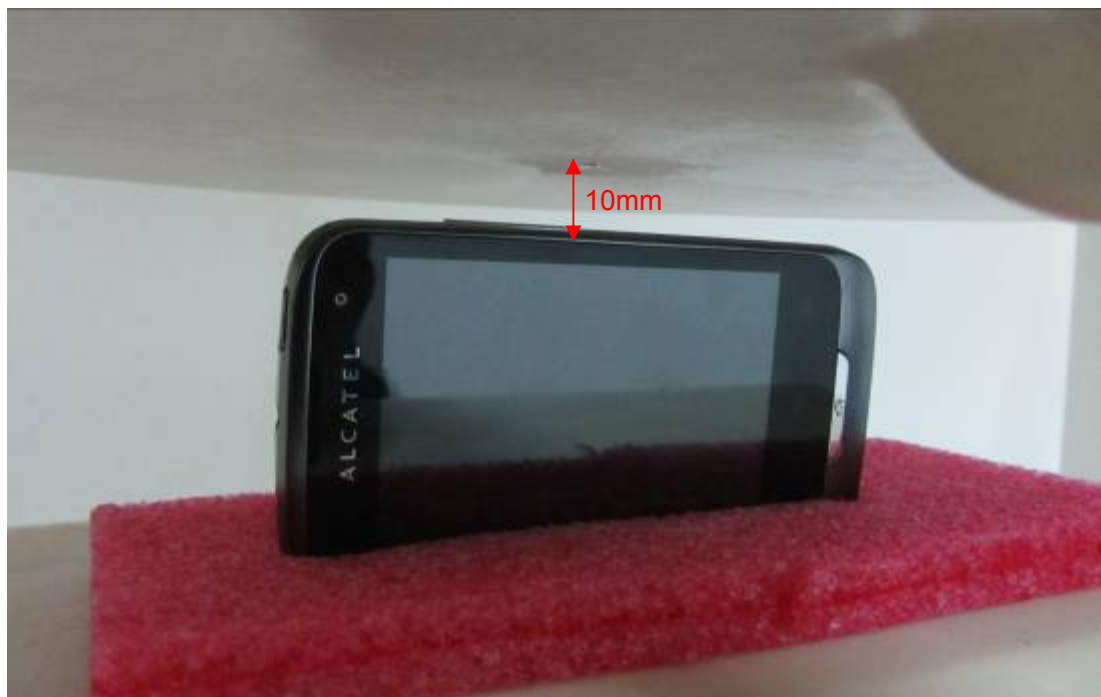
Picture 20: Right Edge, the distance from handset to the bottom of the Phantom is 10mm (Battery 1)
