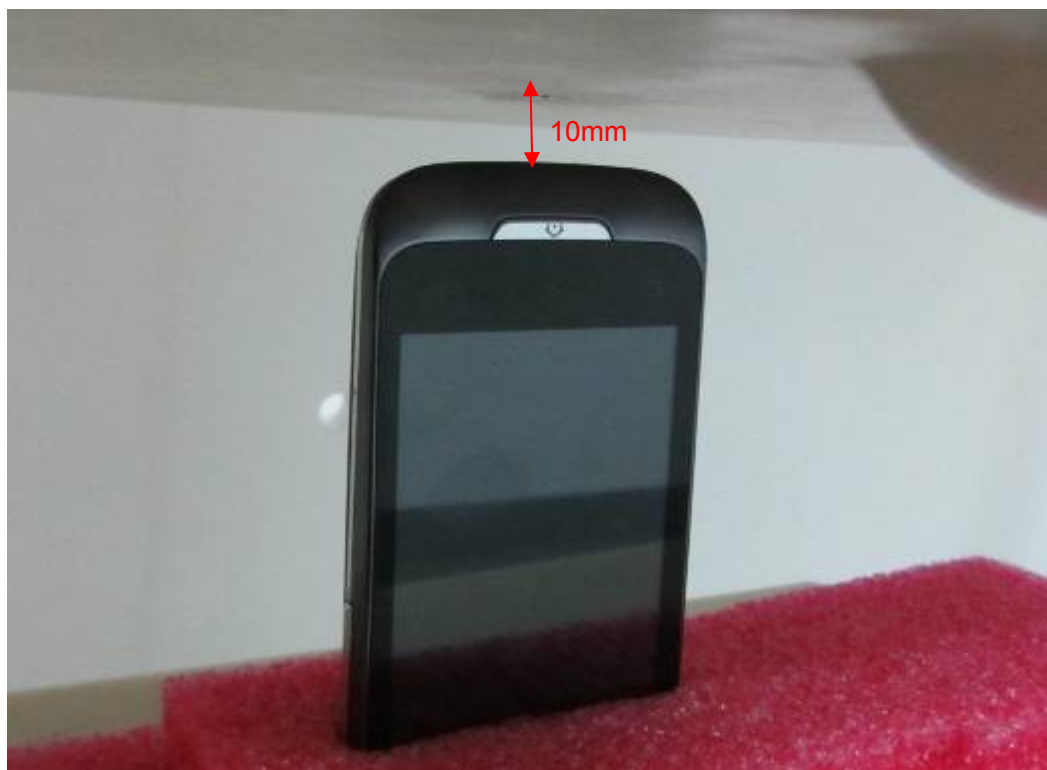
Picture 22: Bottom Edge, the distance from handset to the bottom of the Phantom is 10mm (Battery 1)
