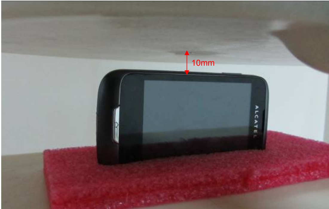
Picture 19: Left Edge, the distance from handset to the bottom of the Phantom is 10mm (Battery 1)
