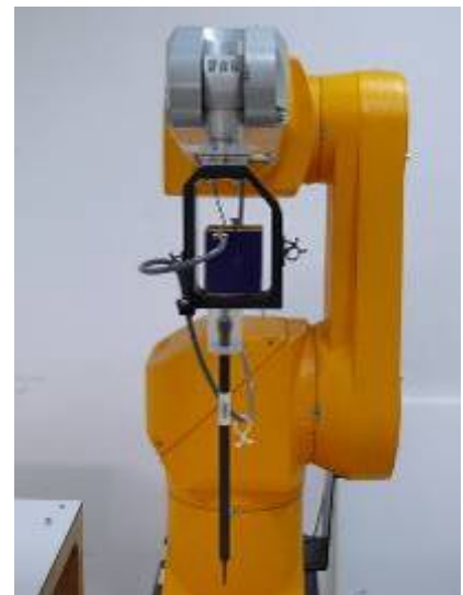
Figure 3. EX3DV4 E-field probe
